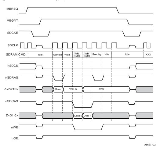
Figure 3-8. SDRAM Write Cycle, Burst of 2
