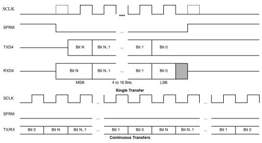
**Note**: The phase and polarity of SCLK can be configured for four different modes. This example shows just one of those modes.
