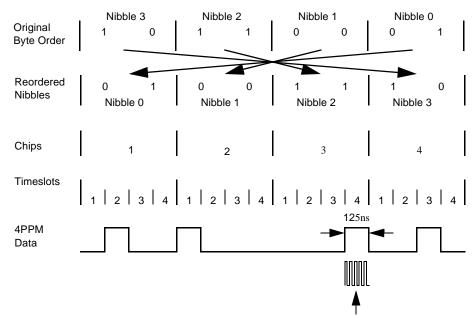
Receive data sample counter frequency = 6X pulse width; each timeslot sampled on third clock.
