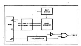
Figure 15. Typical Dot Level Block Diagram
