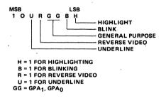
\*More than one attribute can be enabled at the same time. If the blinking and reverse video attributes are enabled simultaneously, only the reversed characters will blink. The 8275H can be programmed to provide visible or invisible field attribute characters.
