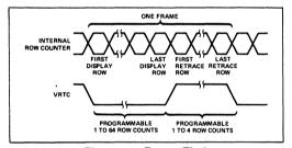
Figure 18. Frame Timing
