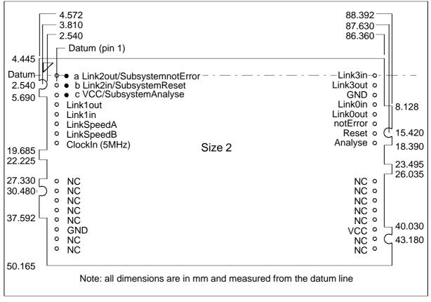
Figure 1.3 PCB profile drawing and pinout
