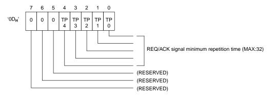
Set the synchronous transfer period for the bus device ID specified by the SEL/RESEL ID register (address  $04_{H}$ ). Note that higher transfer rate than the actual rate may be set if the input clock is high. (ex. 40 MHz: 04h or higher, 30 MHz: 03h or higher, 20 MHz: 02h or higher)
