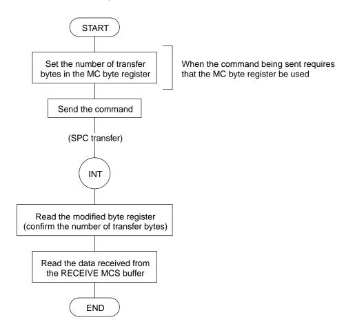
Figure 5.3.1.2 Receive Flowchart for Message, Command, Status Phases
