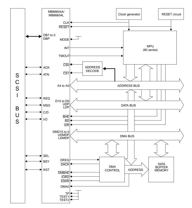
System Configuration Example 1 (80 Series, Separate Bus Type)
