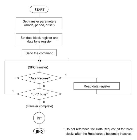
Figure 5.3.2.2 Receive Flowchart for Program Transfer Mode
