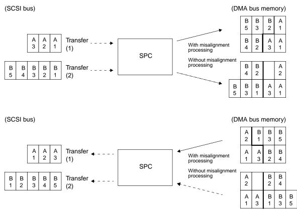
Figure 6.2 DMA Misalignment Processing Example
