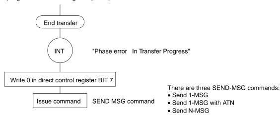
Figure 3.2.3 Transfer Flowchart (Direct Control Register: BIT 7)
