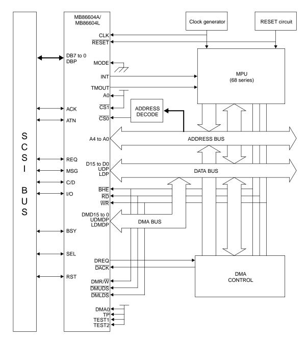
Figure 6.6 System Configuration Example 4 (68 Series, Common Bus Type)
