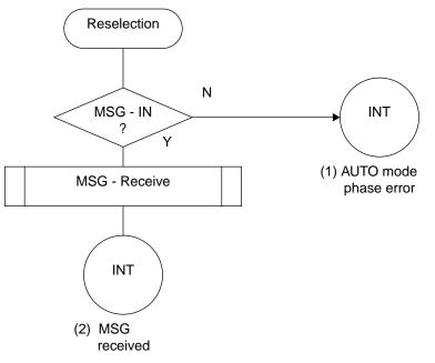
Figure 3.3.4.1 Initiator Automatic Reselection Response Flowchart
