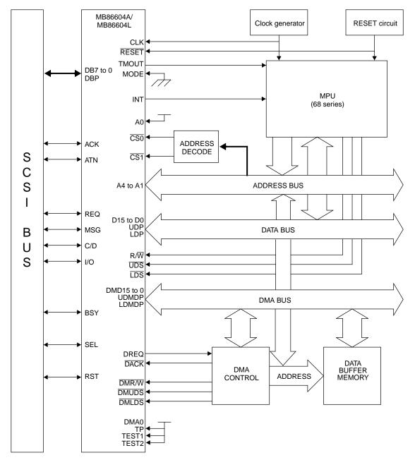
Figure 6.4 System Configuration Example 2 (68 Series, Separate Bus Type)
