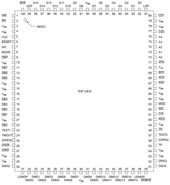
Figure 2.1 MB86604A Pin Assignment Diagram
