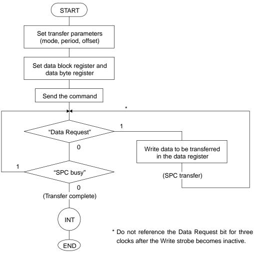
Figure 5.3.2.1 Send Flowchart for Program Transfer Mode
