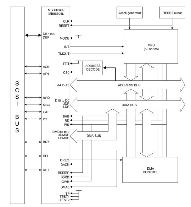
System Configuration Example 3 (80 Series, Common Bus Type)
