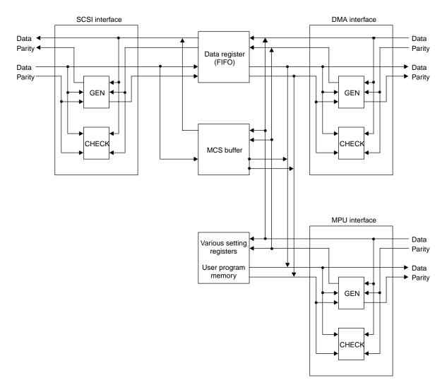
Note: For systems which do not have parity bits on the data bus, respectively pull up or pull down the UDP, LDP pins or the UDMP, LDMP pins with about 10 kiloohms of resistance.
