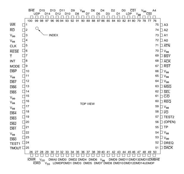
Figure 2.2 MB86604L Pin Assignment Diagram
