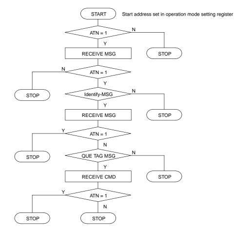
Figure 5.5 Summary Flowchart of Target User Programming Example
