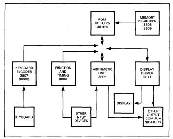
Fig. B-1. PPS-25 Micro-Programmed Processor System
