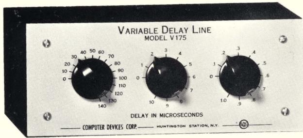
This series of lumped constant Delay Lines is specifically designed for use in the AUDIO and low frequency range (0 to 60 kilocycles). Special "M" section designs, high "Q" coils and temperature compensating capacitors are used to provide minimum phase distortion, low VSWR, low insertion loss and good temperature stability. They are particularly applicable to such sonic, sub-sonic and ultra-sonic uses as:
