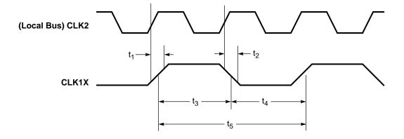
**NOTE:** CLK1X is a divided-down signal from the system's central clock source.
