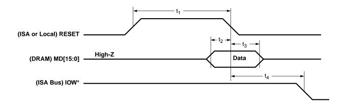
Figure 7-15. Reset Timing
