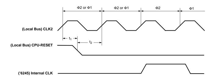
Figure 7-6. Reset Timing (Local Bus)
