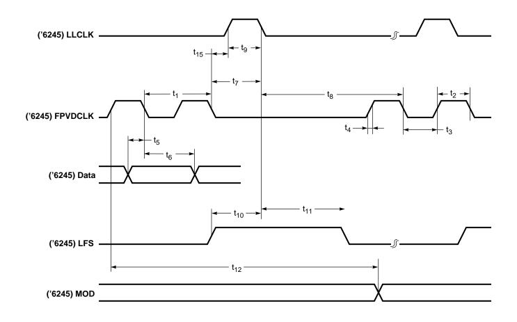
Figure 7-16. STN Monochrome and Color Passive LCD Interface Timing
