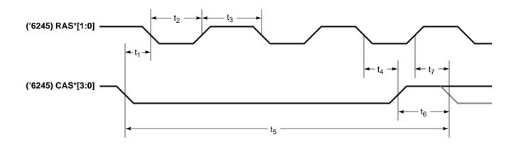
Figure 7-14. CAS\*-before-RAS\* Refresh Timing (Display Memory Bus)
