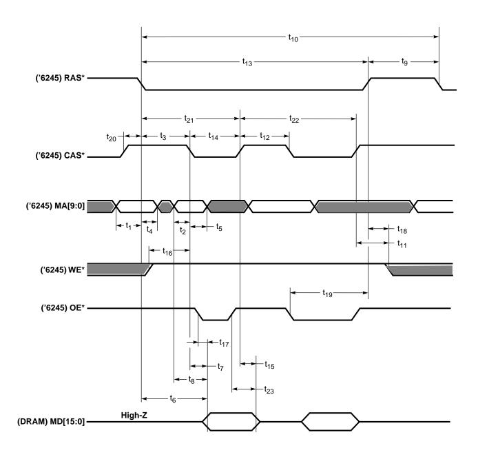
Figure 7-12. Read Timing (Display Memory Bus)
