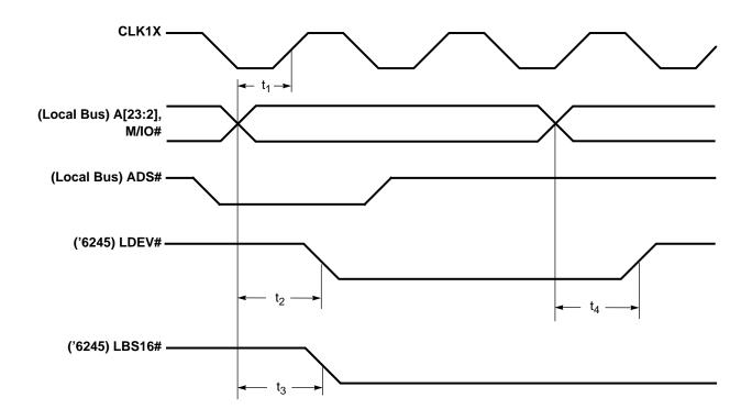
**NOTE:** CLK1X is a divided-down signal from the system's central clock source.
