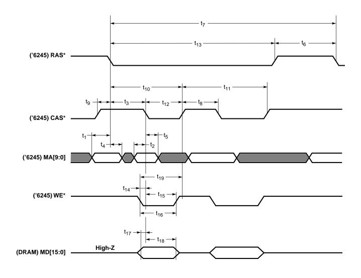
Figure 7-13. Write Timing (Display Memory Bus)
