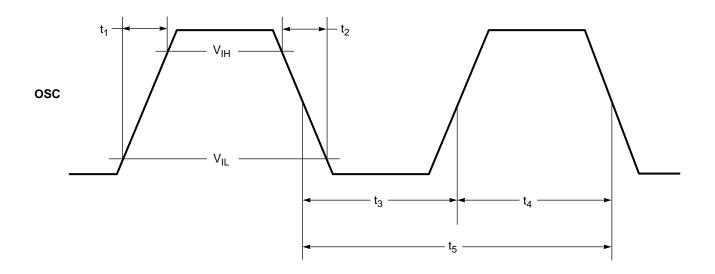
Figure 7-18. Clock Frequency Synthesizer Input
