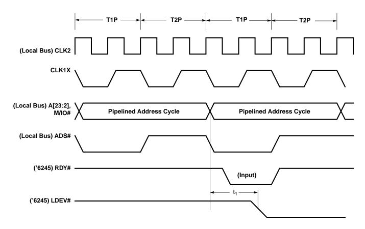
**NOTE:** CLK1X is a divided-down signal from the system's central clock source.
