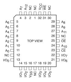
TSOP Top View (8mm x 13.4mm) (T13, H13)
