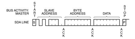
Figure 6. Write Cycle Timing
