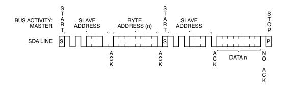
Figure 10. Sequential Read Timing
