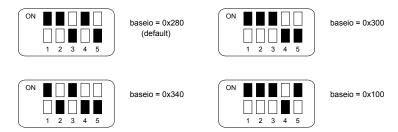
For the multiple DSP32C board, DSP\_MUL, there is also an 8 position dip switch. This selects the base address of the cpu selection register. This register selects which DSP32C PIO is connected to the PC bus at the baseio base address. Some settings for this switch are:
