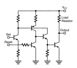
Figure 17. Fast, ECL Flip-Flop
