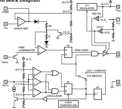
Figure 1. Block Diagram of the AS2842/3/4/5
