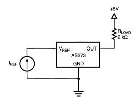
Figure 1. Test Circuit for Output Hysteresis Curve
