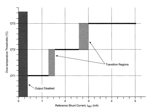
Figure 10. Reference Shunt Current Programming Ranges of Over-temperature Thresholds
