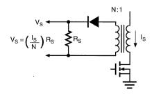
Figure 21. Optional Current Transformer
