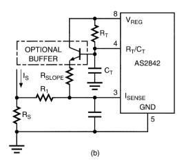
Figure 23. Slope Compensation
