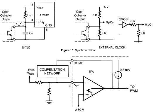
Figure 17. Error Amplifier Compensation
