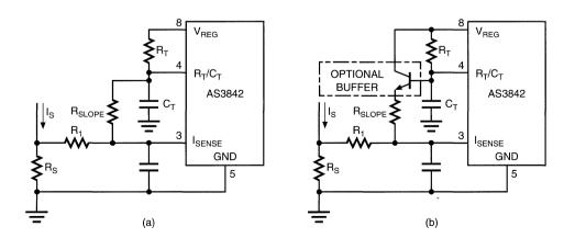
Figure 23. Slope Compensation
