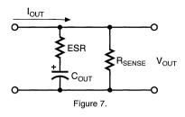
characteristics of the output filter transfer function. The circuit analysis of Figure 7 demonstrates the effects of ESR and  $R_{\text{SENSE}}$ .
