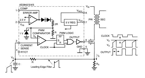
Figure 20. Current Sense/PWN Latch Circuit and Waveforms
