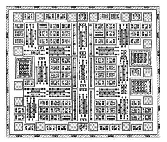
Figure 1. Single Tile Bipolar Array
