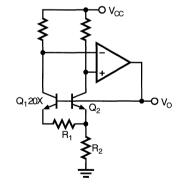
Figure 10. Widlar Band Gap Reference.  $\Delta V_{BE} = V(R3) = V_T * In (A2/A1)$   $V_{OUT} = V_{BE}(Q3) + (R2/R3) * \Delta V_{BE}$
