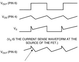
THIS IS THE RESULT OF SUPERIMPOSING  $V_{\rm OS}$  on  $V_{\rm S}.$  This leading edge voltage spike could falsely trigger the current sense comparator and cause noise problem.
