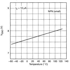
V<sub>EBO</sub> Breakdown Voltage vs Temperature
