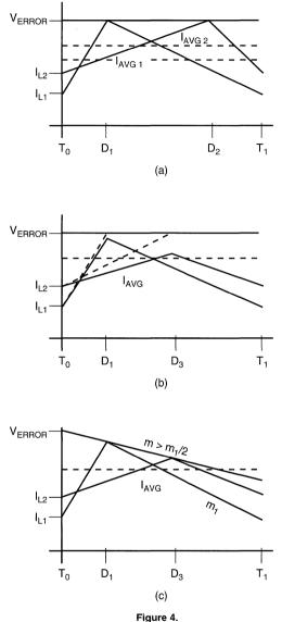
Figure 4a shows the average inductor current  $(I_{AVG 1} \text{ and } I_{AVG 2})$  in dashed lines changes as the duty ratio (D1 and D2) changes. The triangles formed by solid lines represent the actual inductor currents ( $I_{L 1}$  and  $I_{L 2}$ ) at different duty ratios (D1 and D2), and the areas under the triangles are their average currents.
