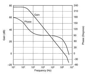
Figure 18. Gain/Phase Response of the AS2842
