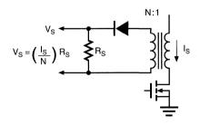
Figure 21. Optional Current Transformer
