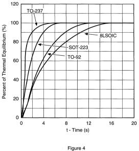
Thermal Response by Package in a Stirred Oil Bath
