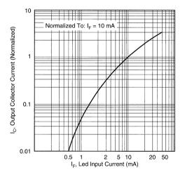
The typical AS3842 maximum  $I_{COMP}$  source current is 800  $\mu$ A. Using Figure 4, and assuming 0.1 CTR at 10 mA diode current, the forward diode current required to generate 800  $\mu$ A of opto-coupler current is 8 mA.
