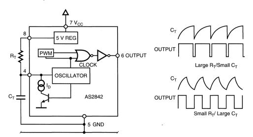
Figure 15. Oscillator Set-up and Waveforms
