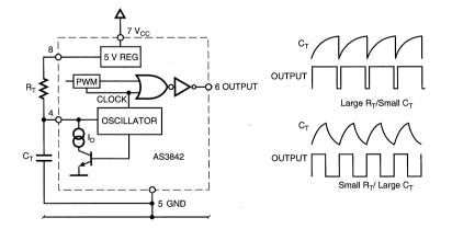
Figure 15. Oscillator Set-up and Waveforms
