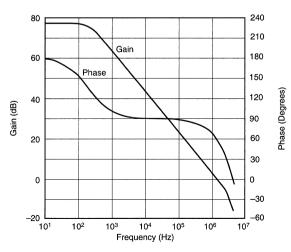
Figure 18. Gain/Phase Response of the AS3842
