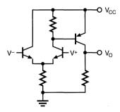
Figure 5. Simple NPN Type Comparator.
