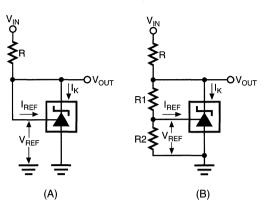
Figure 2. AS431 Precision Voltage Reference A) Fixed B) Programmable
