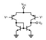
Figure 6. Simple NPN Type Comparator Input Stage.
