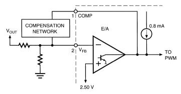
Figure 17. Error Amplifier Compensation
