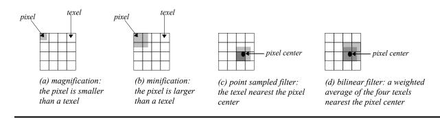
*Magnification* of a texture map occurs when a texture map is "blown up" on screen (see Figure 9.3(a)). For example, if a 64×64 texture map is rendered onto a polygon that covers 128×128 pixels on the screen, an average of four pixels will cover each texel in the texture map, causing noticeable blockiness. The Voodoo Graphics hardware supports bilinear interpolation of texels that greatly reduces the blockiness and pixelization of texture magnification.
