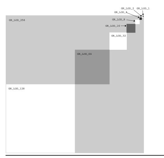
The hardware computes an LOD for every pixel. The integer part of the LOD is used to choose one (or two) of the textures in the current mipmap; the fractional part is used to blend two mipmap levels if desired.
