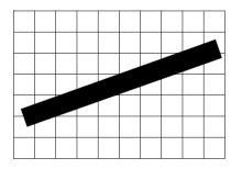
(a) This angled one-pixel wide line segment doesn t cover any pixel completely.
