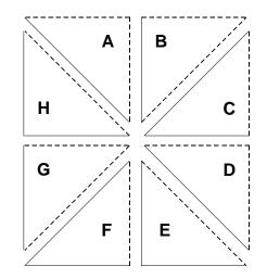
(b) Pixels on solid edges lie inside the triangle; pixels on dotted lines do not. A vertex is inside the triangle (and hence, rendered) if both edges that radiate from it are inside the triangle. Thus, only triangle C will render the center point.
