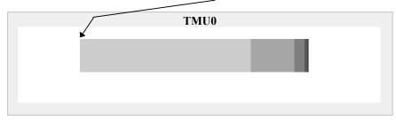
The second scenario loads only the odd LODs. Recall that the largest dimension of odd LODs is an odd power of two. In this case, GR\_LOD\_128, GR\_LOD\_32, and GR\_LOD\_8 are odd LODs.
