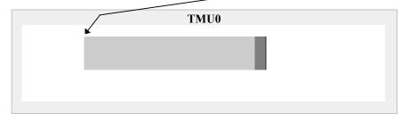
The final scenario loads only the even LODs. Note that no modification is necessary to the values in the GrTexInfo structure pointed to by **info**. Glide will skip over the texture data for the odd LODs, only loading the even ones.
