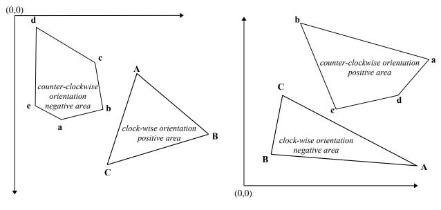
The sign of the area of the triangle can be used for backface culling (quickly discarding triangles that won't be visible on the screen before they are rendered). Because the area must be computed anyway, this is a cheap way to cull. However, removing back-facing triangles earlier may be advantageous. For
