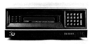
The basic table-top Codex 6030 processor supports 28 terminal ports and is designed for point-to-point data communications networks or for use as a remote concentrator in multi-node networks. The control console features a 32-character LED display, an 18-key arrangement for setting control parameters, and a control switch which can only be operated with a key.
