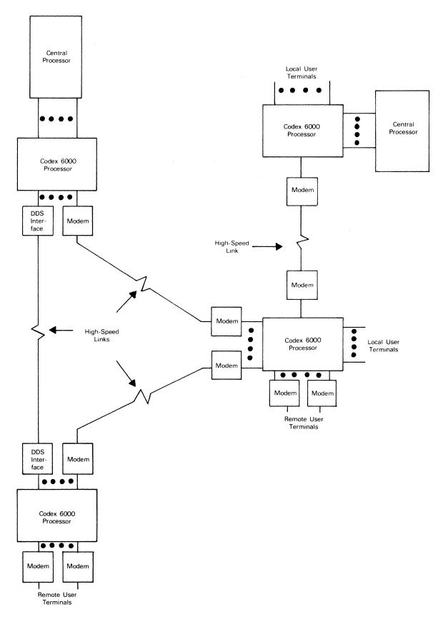
Figure 1. Typical network configuration employing Codex 6000 Intelligent Network Processors.
