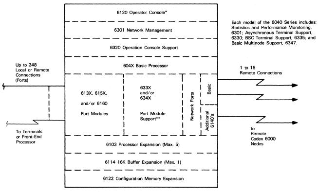
\*At least one 6120 Operator Console is required in a network.
