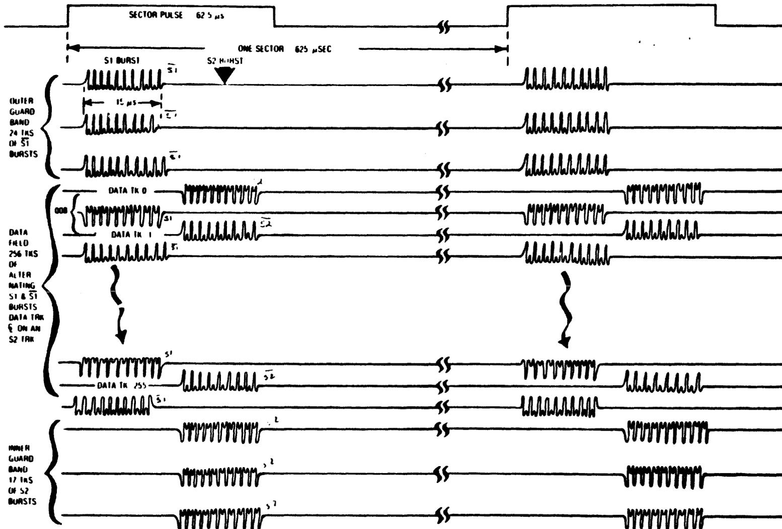
Figure 1 RL01 Servo Data Format
