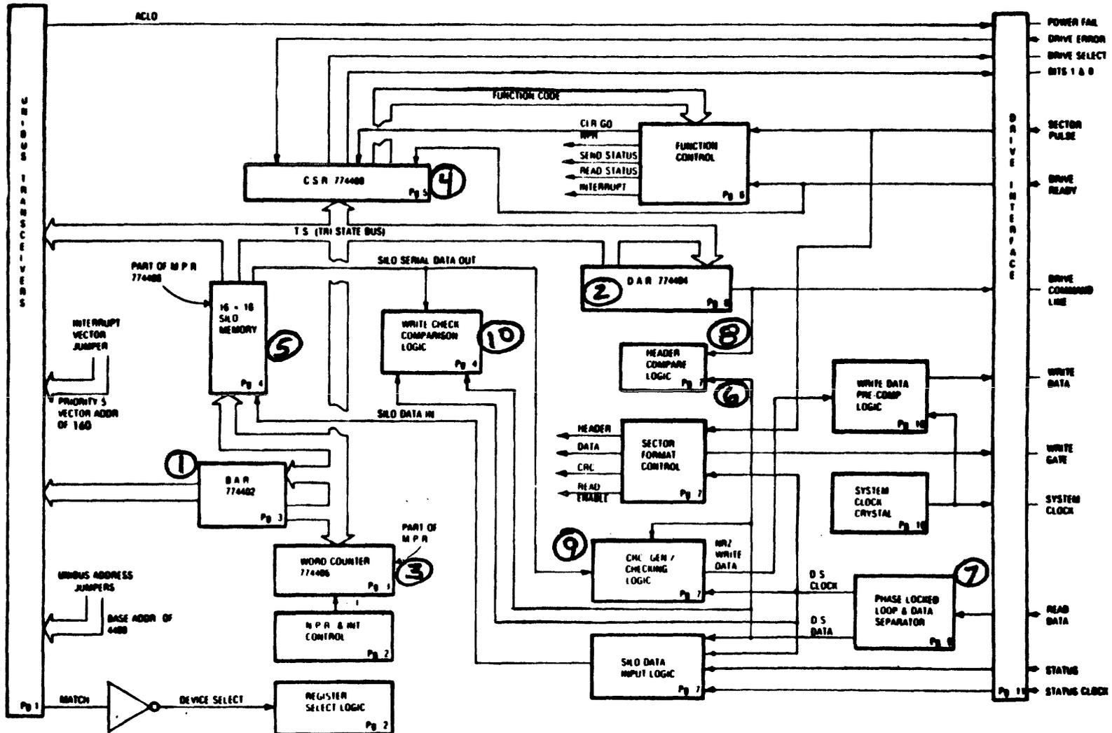
Figure 7 M7762 RL11 Basic Block Diagram
