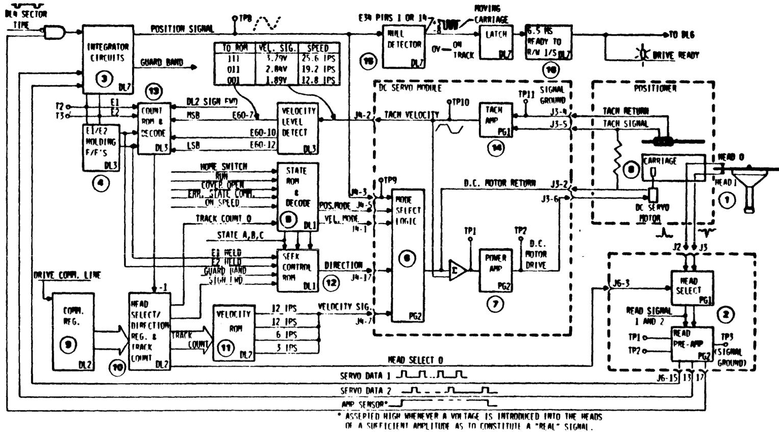
Figure 2 Track — Following Servo Block Diagram
