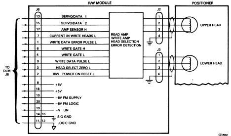
Figure 2-4 Signal and Function Diagram of R/W Module, R/W Heads
