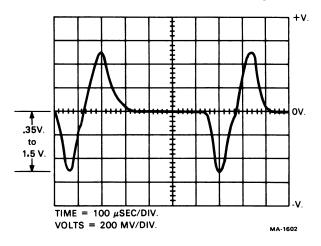
Figure 9-1 Sector Transducer Output
