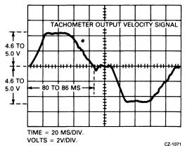
Figure 9-10 Tachometer Output Velocity Signal
