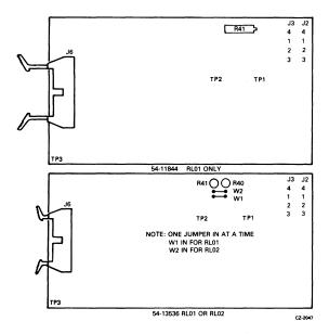
Figure 2-10 R/W Module Layout — Top View
