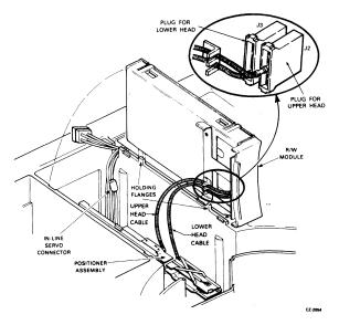
Figure 9-3 Positioner and Read/Write Module Box Assembly
