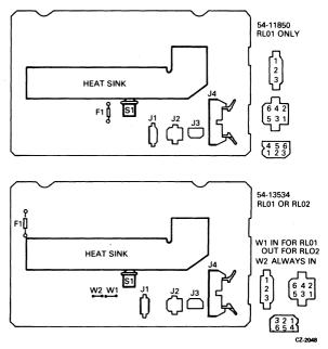
Figure 2-12 DC Servo Module Layout — Bottom View
