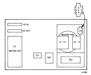
Figure 2-11 Power Panel Layout — Front View
