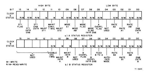
Figure 3-1 KW11-K A and B Register Formats
