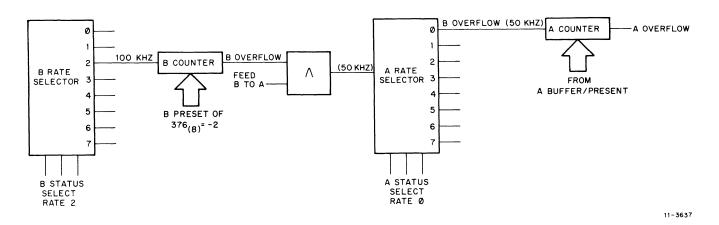
Figure 2-2 Feed B to A Block Diagram
