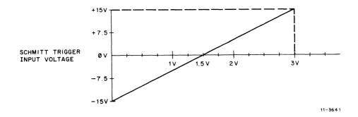
Figure 2-6 Input and Threshold Input Voltage Relationship
