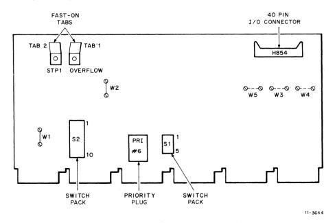
Figure 2-9 M7025 Module Component Locations
