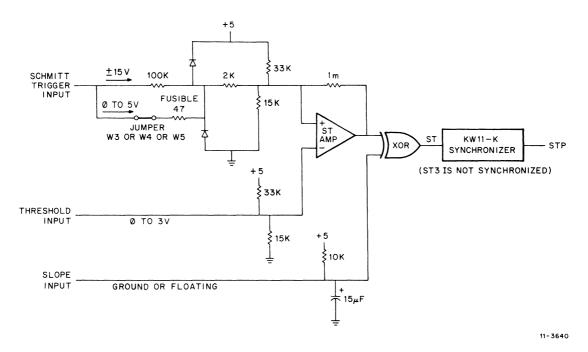
Figure 2-4 Schmitt Trigger Circuitry
