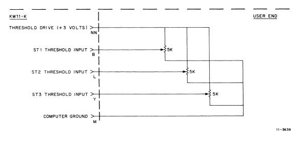
Figure 2-5 Threshold Control
