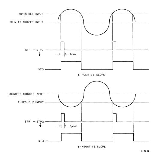
Figure 2-7 Schmitt Trigger Slope Relationship
