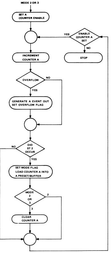
Figure 2-1 Clock A Mode Flow Diagram
