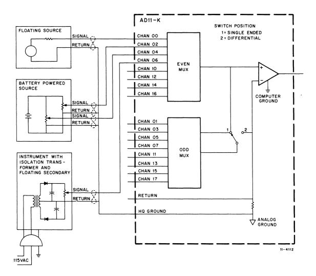
Figure 2-3 Floating AD11-K Input Signals
