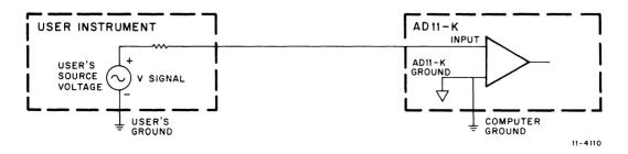
Figure 2-2 AD11-K Input Referenced to User's Ground
