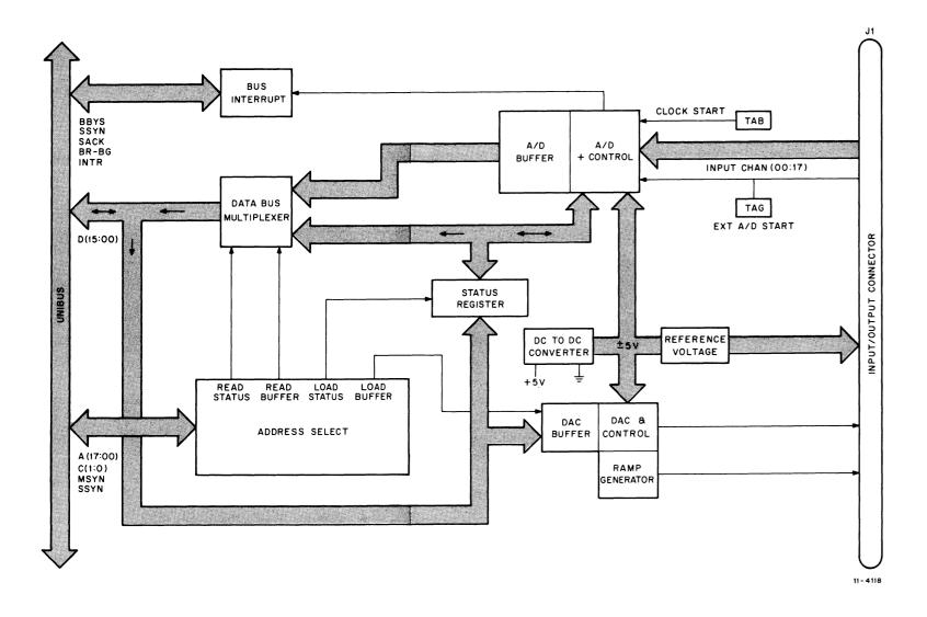
Figure 1-1 AD11-K Block Diagram
