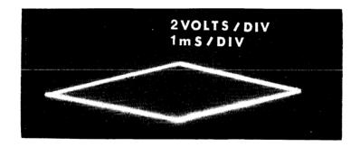
FIGURE 4-11 COARSE DATA PHASE DETECTOR INTEGRATOR OUTPUT (IN LOCK CONDITION)
