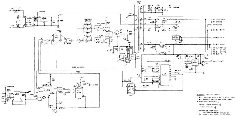
\* FOR 448-FPC, CR6 TO BE REPLACED BY JUMPER, CR6 TO BE DELETER, R41 TO BE BB.7 K, 1%, R42 TO BE 5.3 MEG, 5%.
