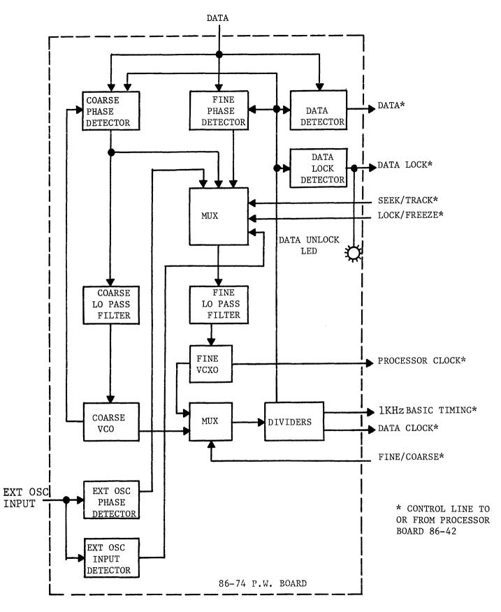
FIGURE 4-5 BASEBAND DATA PHASE LOCK BLOCK DIAGRAM, MODEL 468-DC
