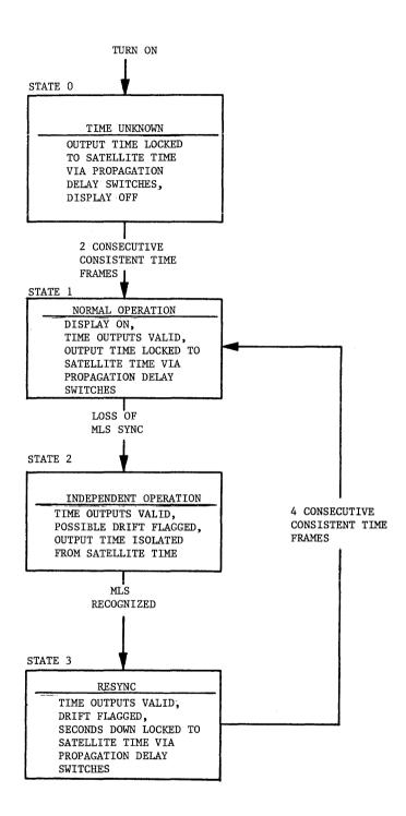
FIGURE 4-19 FRAME SYNC CONTROL STATE DIAGRAM
