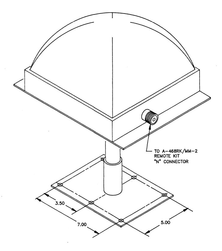
MODEL A-468MS/RK/MM-2 GOES ANTENNA WITH MOUNTING HARDWARE
