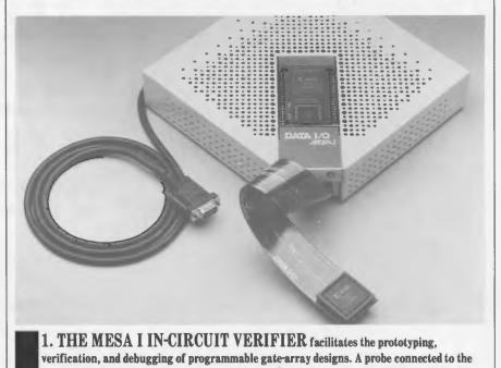
chassis by a flex-circuit cable plugs into the array's socket in the target system and, in turn, holds the chip being debugged.
