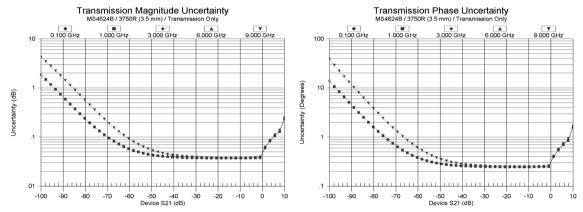
Transmission Measurements: 3.5 mm Connectors
