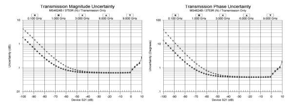
Transmission Measurements: N Connectors
