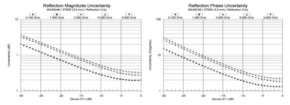
Reflection Measurements: 3.5 mm Connectors
