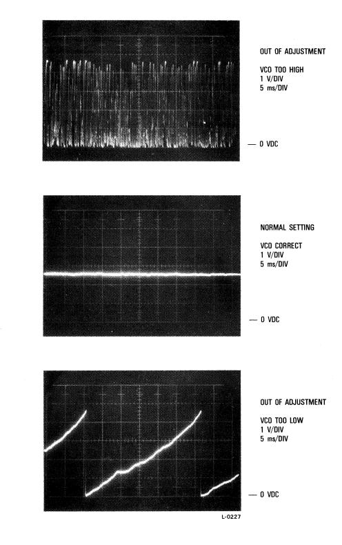
Figure 6. Typical 5 Mb/s Data Bit-Sync Adjustment Waveforms (TP4)
