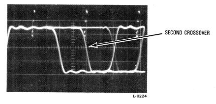
B. SYMMETRY CORRECTLY ADJUSTED
