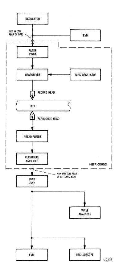
Figure 8. Direct Record/Reproduce System Test Setup
