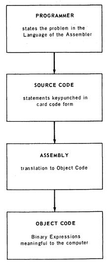
Figure 1-1. Source-to-Object Code Translation with Assembler
