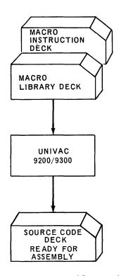
Figure A-1. Schematic of Preassembly Macro Pass Operation
