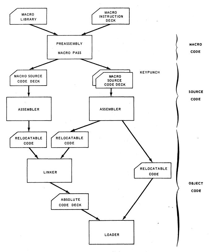
Figure 1-2. UNIVAC 9200/9300 Assembly System
