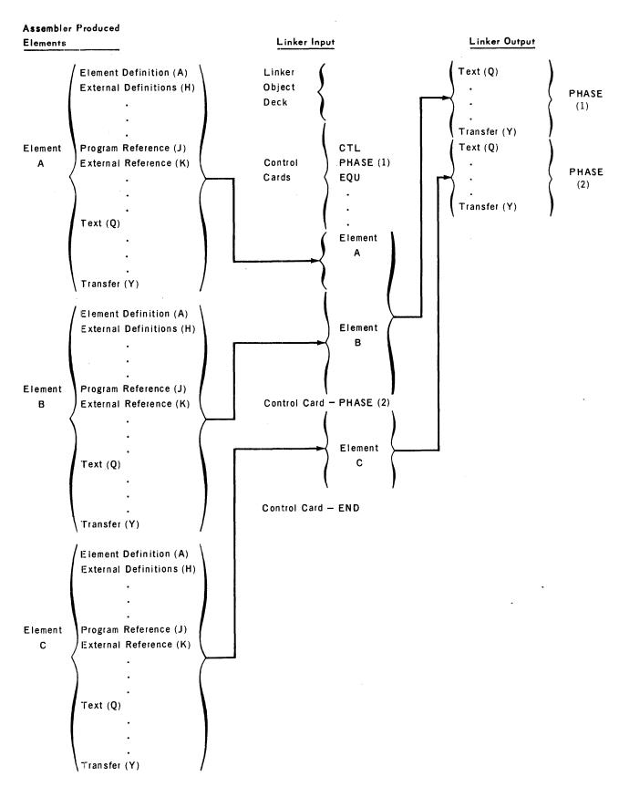
Figure 5-6. Linker Input Deck Sequence for Two-Pass Operation
