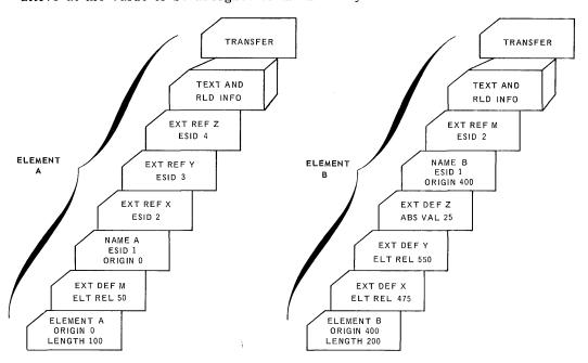
Figure 5-1. Elements A and B Deck Structure
