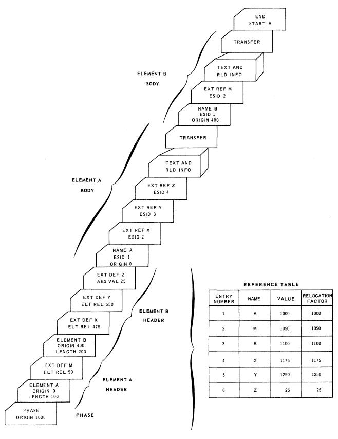
Figure 5-3. Header Processing
