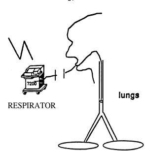
Figure 4-7: Increased Peak Pressure and Decreased Tidal Volume Caused by a Kinked Tube
