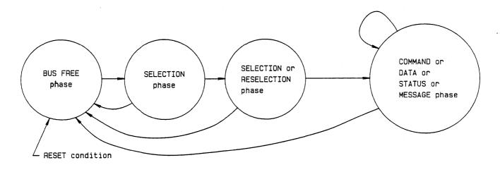
FIGURE 5-2. Phase Sequences with Arbitration
