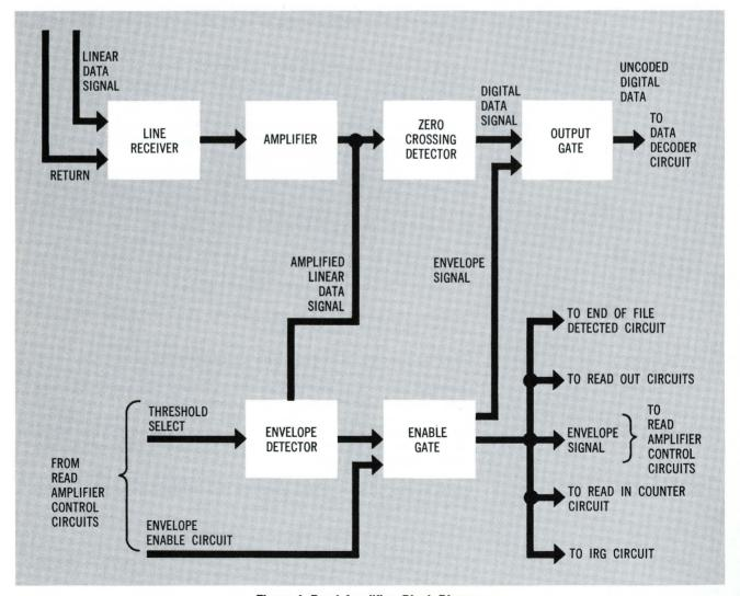
Figure 4. Read Amplifier, Block Diagram
