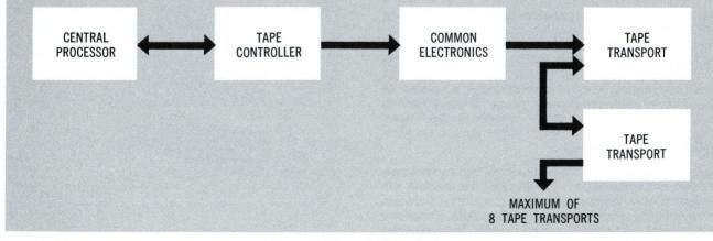
Figure 2. Magnetic Tape System
