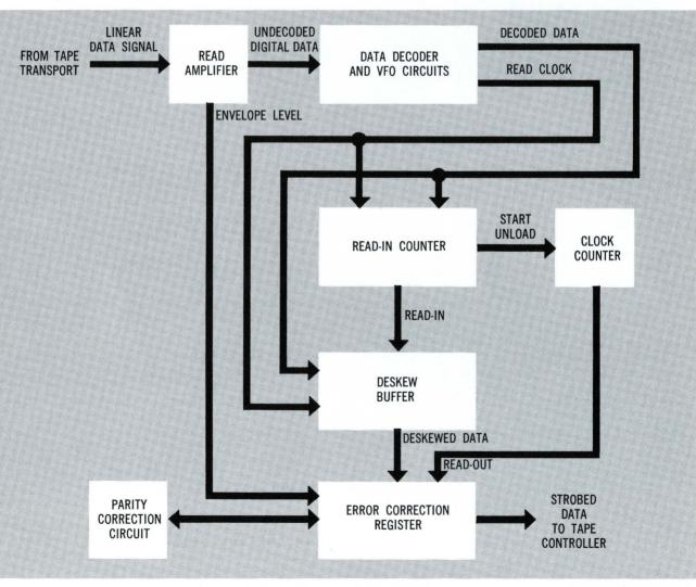
Figure 3. Read Circuits, Block Diagram
