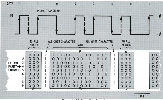
Figure 1. PE Recording Format
