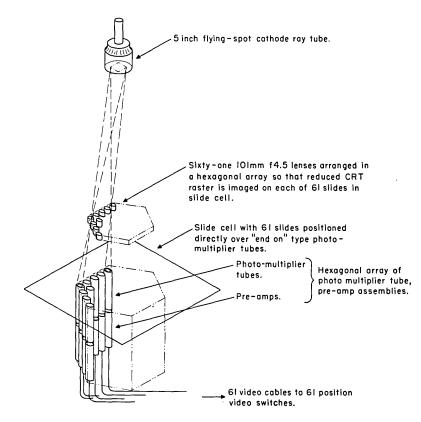
Fig. 2. The 61-slide, simultaneous scanner for PLATO II
