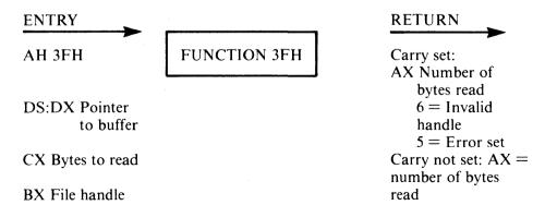
Function 3FH transfers count bytes from a file into a buffer location. It is not guaranteed that all count bytes will be read. For example, reading from the keyboard will read at most one line of text. If the returned value is zero, then the program has tried to read from the end of file. All I/O is done using normalized pointers; no segment wraparound will occur.
