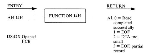
Function 14H reads the next record in a sequence of records. DX must contain the offset (from the segment address in DS) of an opened FCB. The record pointed to by the current block (offset 0CH) and Current Record (offset 20H) fields is loaded at the Disk Transfer Address, then the Current Block and Current Record fields are incremented.
