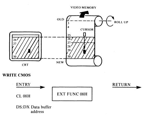
Extended 08H writes up to 512 bytes to CMOS RAM (battery back-up memory). The data to be written is stored in an I/O buffer addressed by registers DS and DS. The format of the buffer is as follows.
