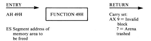
Function 49H returns a piece of memory to the system pool that was allocated by the Allocate Memory function.
