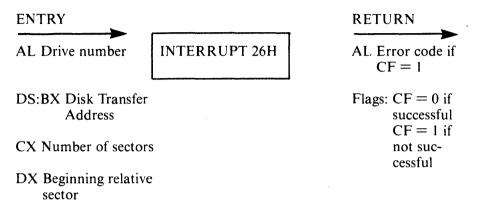
Interrupt 26H transfers control directly to the MS-DOS I/O System for a disk write.
