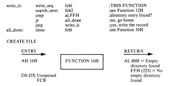
Function 16H searches a disk directory for an empty entry or an entry for a specified filename. DX must contain the offset (from the segment address in DS) of an unopened FCB. The directory is then searched for the specified entry.
