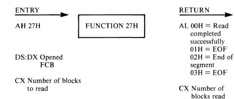
Function 27H reads a specified block of records. DX must contain the offset (to the segment address in DS) of an opened FCB. CX must contain the number of records to read. If it contains 0, the function returns without reading any records (no operation). The specified number of records — calculated from the Record Size field (offset 0EH) — is read starting at the record specified by the Relative Record field (offset 21H). The records are placed at the Disk Transfer Address.
