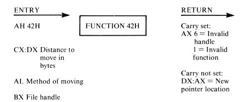
Function 42H moves the read/write pointer according to one of the following methods.
