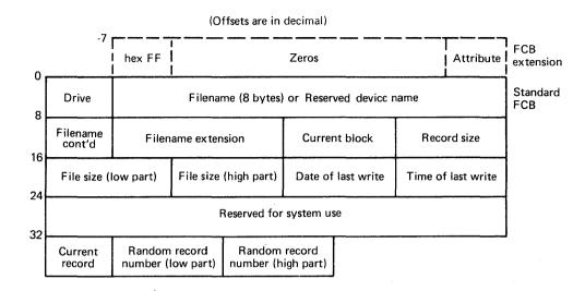
Unshaded areas must be filled in by the using program. Shaded areas are filled in by the DOS and must not be modified.
