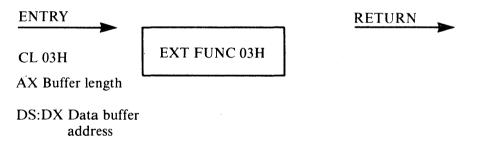
Extended Function 03H sounds the beep tone on the APC. The I/O buffer addressed by registers DS and DX contains beep data. Register AX is set to the I/O buffer length in bytes.
