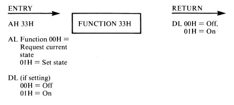
MS-DOS ordinarily checks for a CTRL-C on the controlling device only when doing function call operations 01H-0CH to that device. Function 33H allows you to expand this checking to include any system call. For example, with the CTRL-C trapping off, all disk I/O will proceed without interruption. With CTRL-C trapping on, the CTRL-C interrupt is given at the system call that initiates the disk operation.
