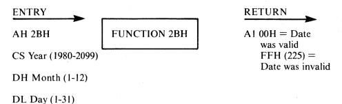
Function 2BH sets the system date. Registers CX and DX must contain a valid date in binary.
