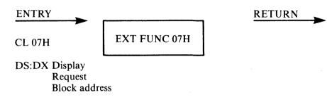
Extended Function 07H allows the assembly language programmer to perform high speed block level I/O operations to the console through the DMA. Five different operations may be performed through this function. They are identified by the command number passed in the Display Request Block. The Extended Function 07H commands are listed in Table 3-6.
