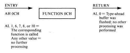
Function 0CH empties the keyboard type-ahead buffer. Further processing depends on the value in AL when the function is called.
