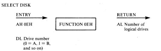
Function 0EH allows for selecting a default disk drive. The drive specified in DL (0A, 1B, and so on) is selected as the default disk. The number of drives is returned in AL.
