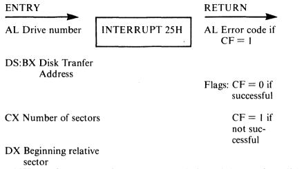
Interrupt 25H transfers control directly to the MS-DOS I/O System for a disk read.
