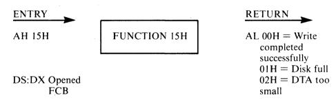
Function 15H writes the next record in a sequence of records. DX must contain the offset (from the segment address in DS) of an opened FCB. The record pointed to by Current Block (offset 0CH) and Current Record (offset 20H) fields is written from the Disk Transfer Address, then the current block and current record fields are incremented.
