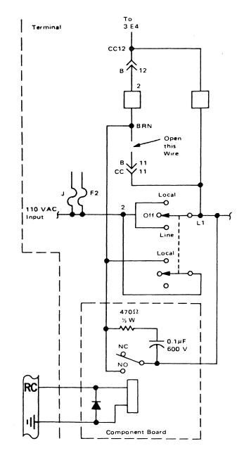
TTY Terminal Schematic Incorporating Automatic Reader Control
