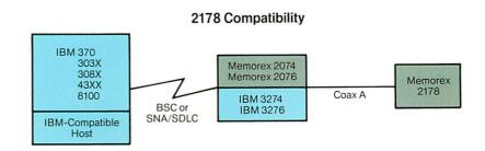
environment. It simply plugs into a Memorex 2074 or 2076 Cluster Controller, or an IBM 3274 or 3276 Cluster Controller.
