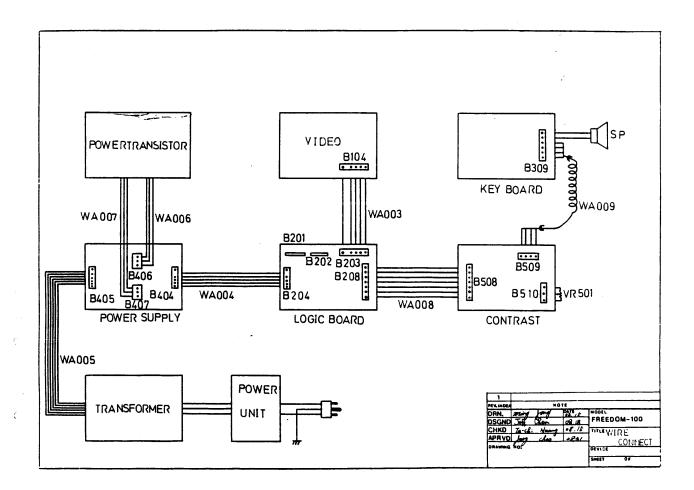
Internally, the Freedom 100 consists of a Transformer and Voltage Selector Switch for converting 115V or 230V AC main power to 10.5V AC, 16.7V AC, and 21.3V AC.
