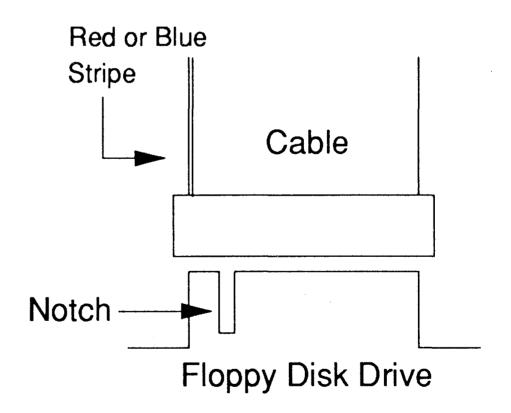
**WARNING!** Connecting this cable backwards may cause irreversible damage!
