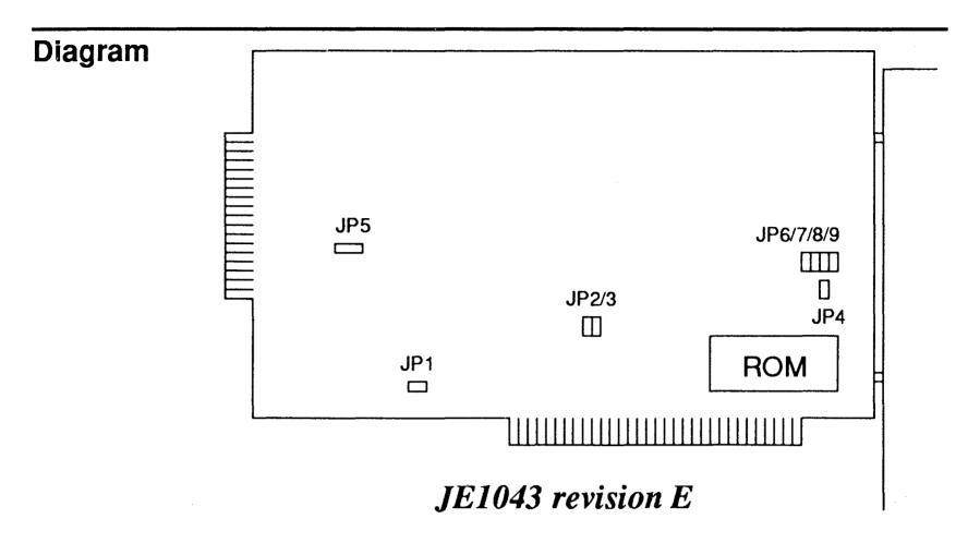
**NOTE:** Some versions of the JE1043 do not have JP6 through JP9 labeled on the board. Instead they are labeled "DIP SW1". If you have received this version, refer to the following figure. There are no functional differences between the two versions.
