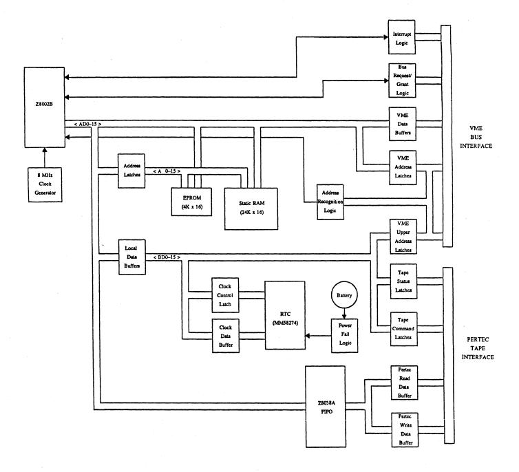
Figure 1-1. VME-TC50 Block Diagram
