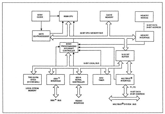
Figure 1. iSBC® 386/21/22/24/28 CPU Board Block Diagram
