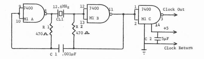
Figure 5-16. Line Lock Oscillator Schematic
