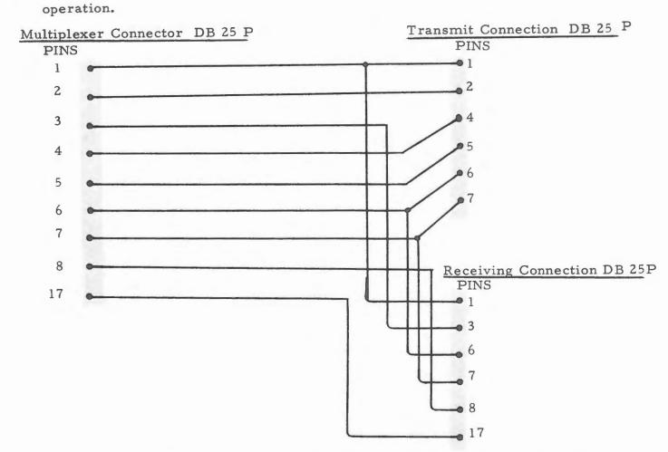
Multiplexer to FDT synchronous or asynchronous controller, HALF Duplex operation.
