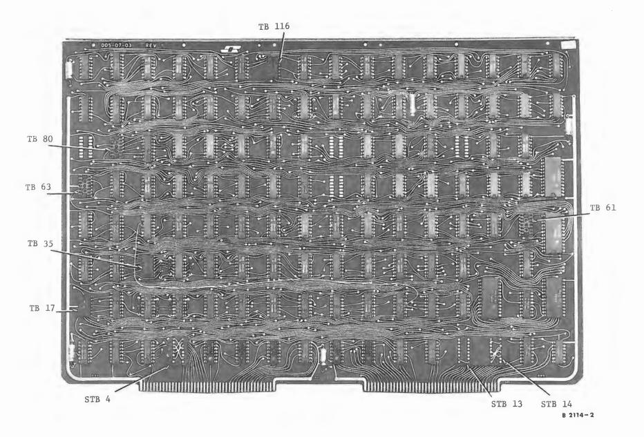
Figure 5-4. Data Control Circuit Module
