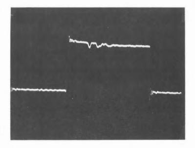
Location: Collector of inhibit transistor MEL Volts/Div: 0.5 x 10 Time/Div: 0.2 microseconds
