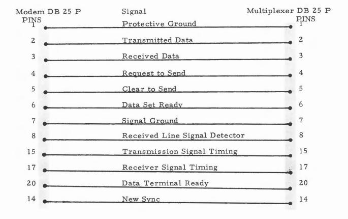
Modem to Multiplexer, full or half duplex operation. Reference standard I/O cable drawing 001-10-13.
