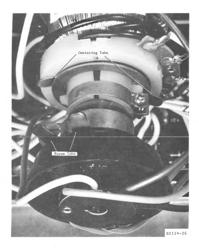
Figure 7-7. Cathode Ray Tube Adjustments
