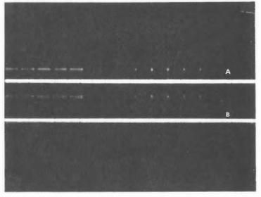
Location: Pins 6 & 8 M13 Split Screen Volts/Div: A 0.5 x 10 B 0.5 x 10 Time/Div: 0.1 milliseconds
