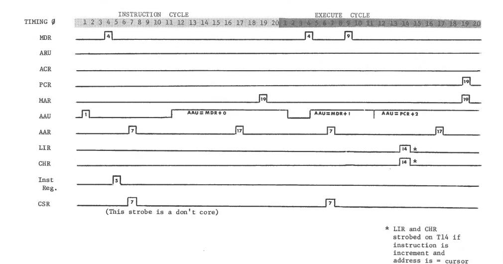
Figure 4-5. System Timing Example, Increment and Store Instruction
