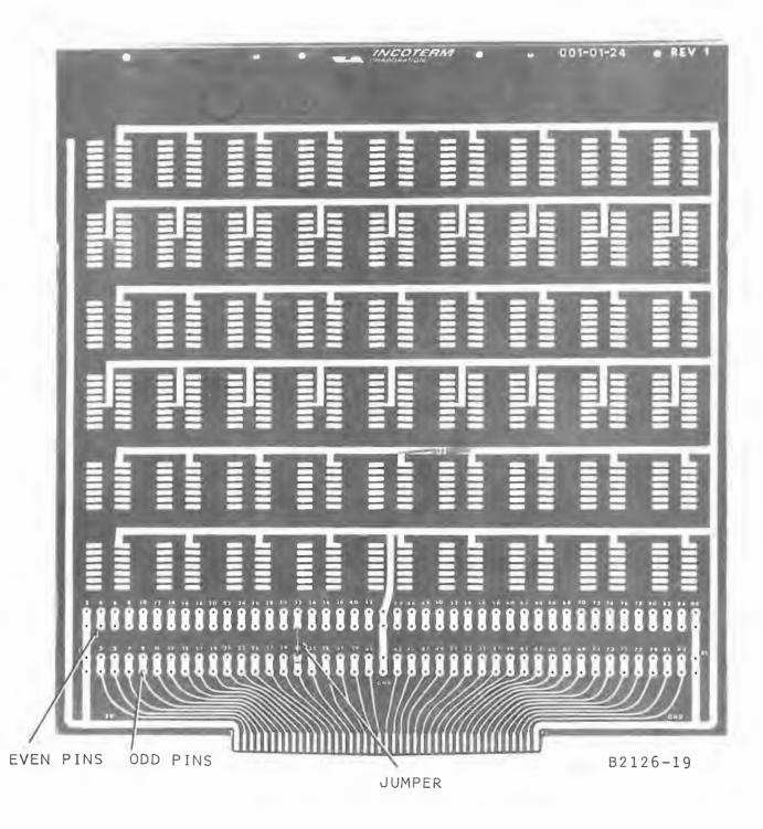
Figure 1. Dummy Controller
