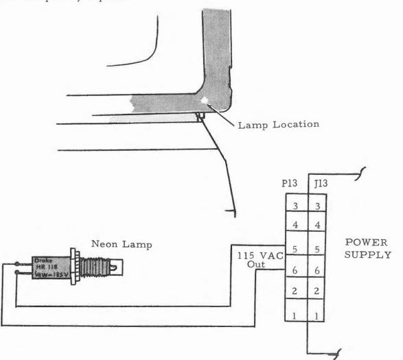
Figure 1. Optional Neon Lamp Power Indicator with Power Supply Connections
