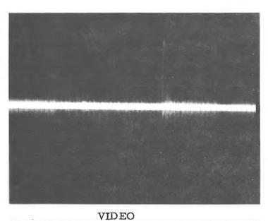
Location: Pin 8 M7 RMTU Volts/Div: 0.2 x 10 Time/Div: 10 microseconds
