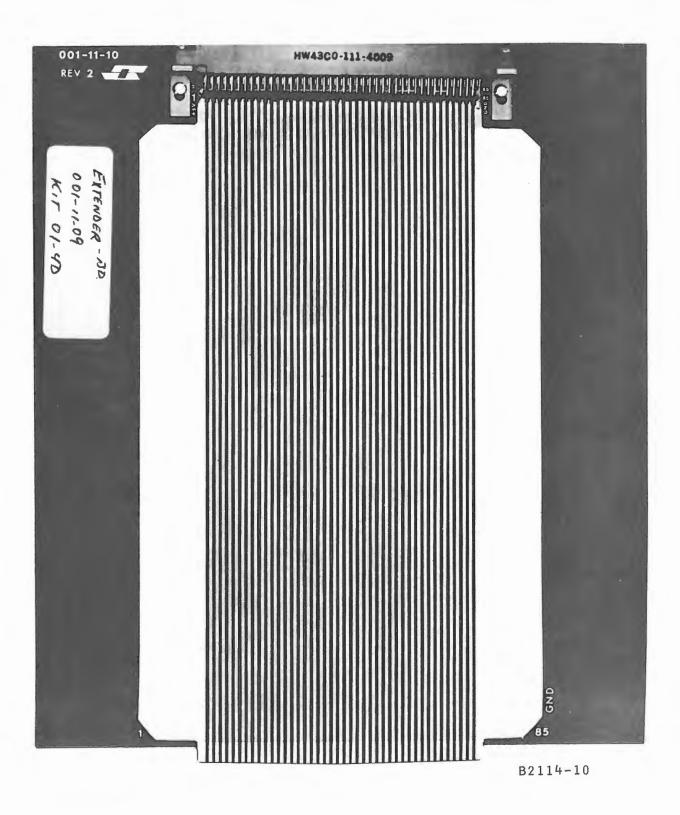
Figure 7-4. Controller Circuit Board Extender
