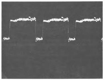
Location: Pin 1 M40 RMTU Volts/Div: 0.2 x 10 Time/Div: 0.5 microseconds
