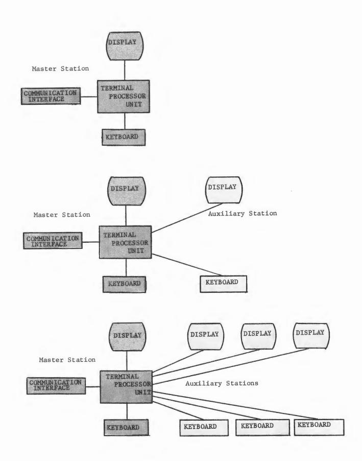
Figure 1-1. Minimum Terminal Configurations
