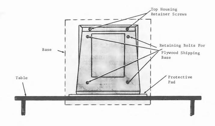
Figure 2-2. Removal of Plywood Base
