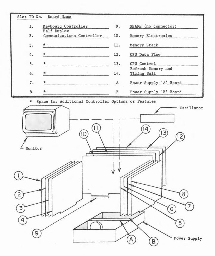
Figure 2-3. Circuit Board Identification and Location
