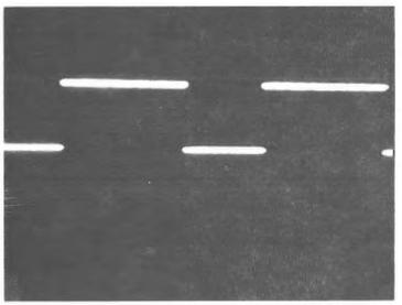
Location: Pin 11 M45 RMTU Volts/Div: 0.2 x 10 Time/Div: 0.1 milliseconds
