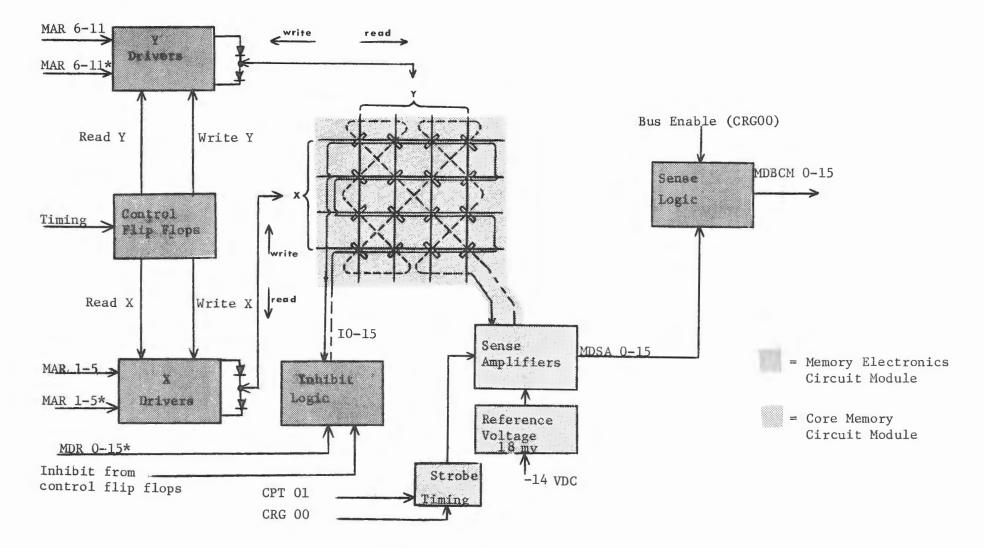
Figure 5-9. Simplified Block Diagram, Memory System
