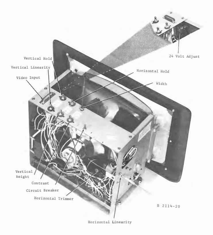
Figure 7-6. T.V. Monitor Adjustments
