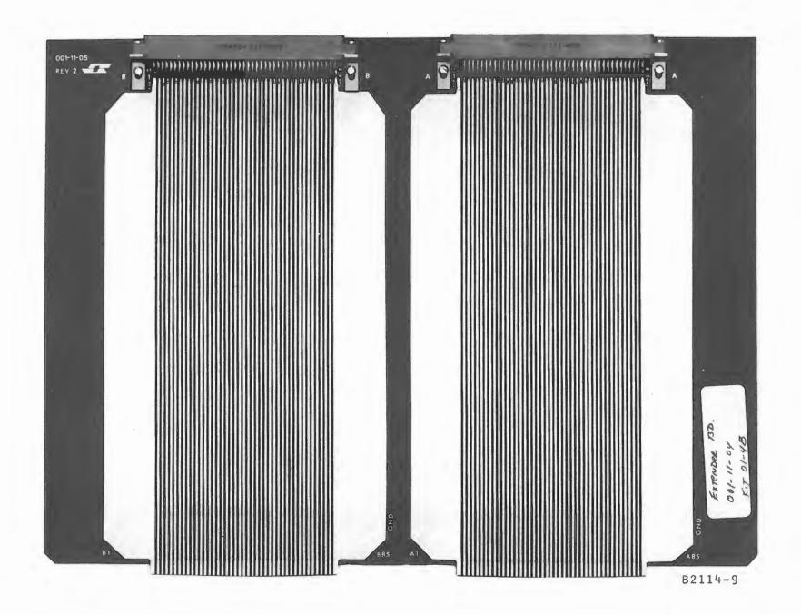
Figure 7-5. Computer Circuit Board Extender
