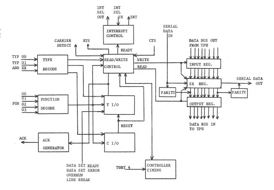
Figure 6-6. Block Diagram Asynchronous Controller
