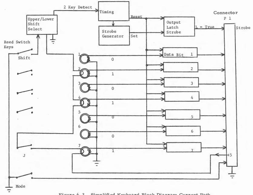
Figure 6-2. Simplified Keyboard Block Diagram Current Path Illustrated for J Key
