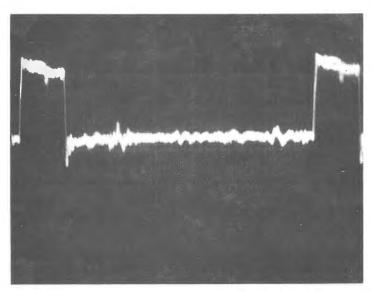
Location: Pin 10 E9 Mem Stack Volts/Div: 0.2 x 10 Time/Div: 0.2 microseconds
