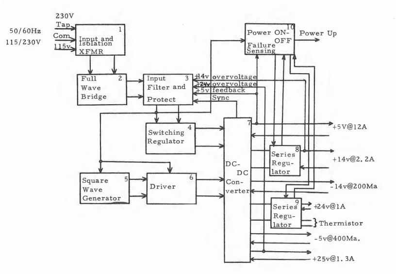
Figure 2. Power Supply Block Diagram
