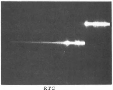
Location: Pin 12 M94 RMTU Volts/Div: 0.2 x 10 Time/Div: 5 milliseconds
