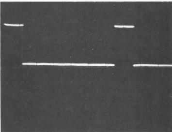
Location: Pin 6 M20 RMTU Volts/Div: 0.2 x 10 Time/Div: 10 microseconds
