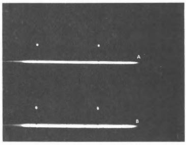
Location: Pins 6 & 8 M18 Split Screen Volts/Div: A 0.5 x 10 B 0.5 x 10 Time/Div: A & B 5 milliseconds
