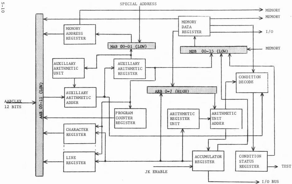
Figure 5-2. Simplified Block Diagram TPU Data Flow
