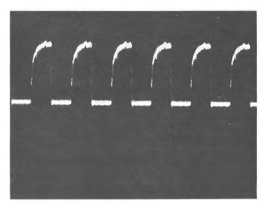
Location: Pin 12 M108 RMTU Volts/Div: 0.2 x 0 Time/Div: 1.0 microseconds
