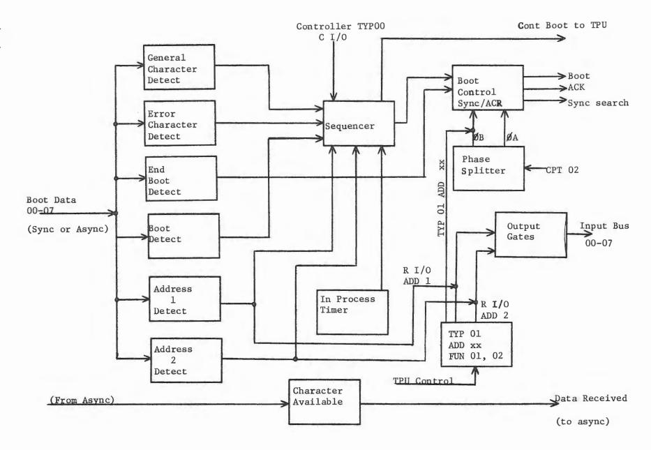
Figure 6-11. Simplified Diagram Boot Controller
