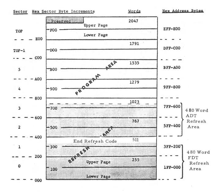
Figure 1. 2K Core Memory Layout Illustrating FDT and ADT Refresh Area For Alternate Line Operation.
