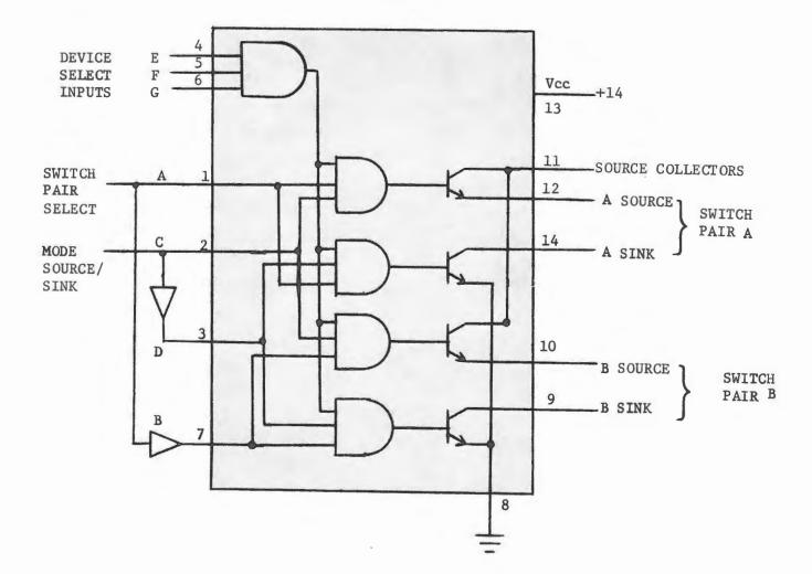
Figure 5-10. Simplified Functional Diagram and Logic Table for SN 75324 Memory Driver
