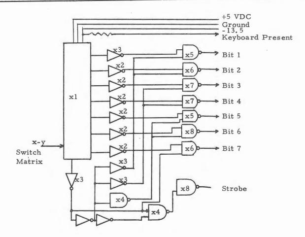
Figure 3. Simplified Block Diagram Keyboard Electronics With Read Only Memory
