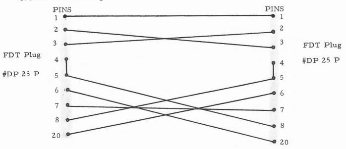
Half duplex operation directly connecting two free standing displays. Reference cable drawing 001-10-92. This cable for asynchronous operation only.
