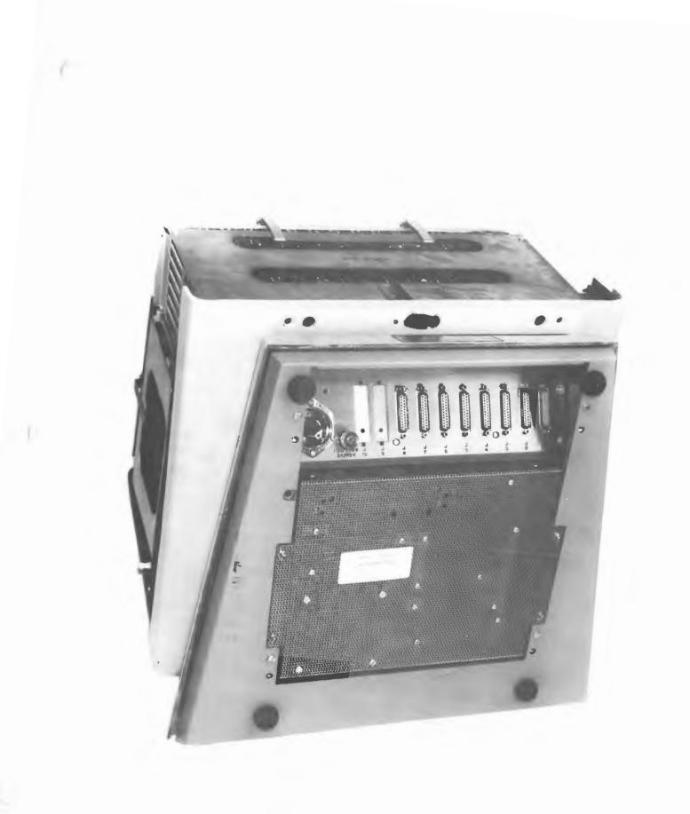
Figure 1. Bottom View Model 010 Terminal System Power Supply
