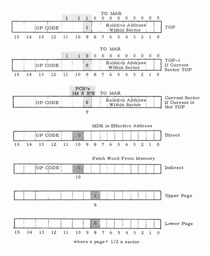
Figure 4-4. Effective Address Calculation Illustrated
