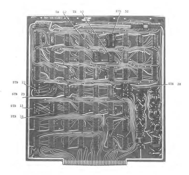
Figure 6-7. Synchronous Controller
