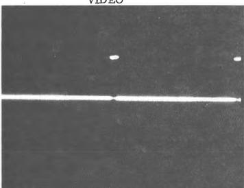
Location: Pin 15 M45 RMTU Volts/Div: 0.2 x 10 Time/Div: 0.1 milliseconds
