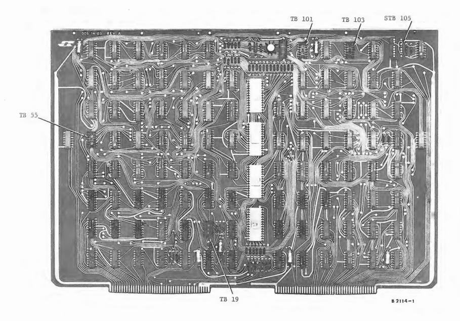
Figure 5-12. Refresh Module Timing Unit
