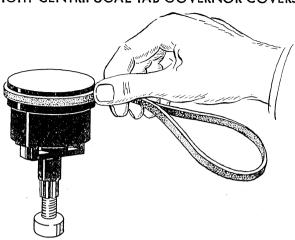
Mr. E. W. Trueblood, Customer Engineer of the Terra Haute Branch Office has suggested a method for easy removal of the former smooth centrifugal governor cap. Wayne suggests that a V-Belt turned wrong side out and held tightly around the cover, as illustrated, greatly aids in removing tight caps. Governor caps on new ET¹s have serrations to reduce difficulty in removal of tight caps.
