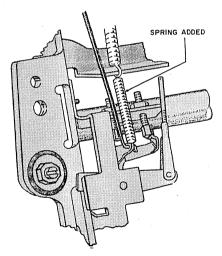
This may be helpful in correcting certain space bar operations where insufficient cam pressure is a problem and particularly for those cases where the ET is in a cold location. This procedure should be used only when all other adjustments and parts are found correct.
