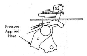
In News Letter #43 a procedure was presented for improving touch on Model B Standard ET's. Another method for improving touch which has been used successfully in several Branch Offices is that of flexstoning the edge of the nylon cam as shown in the accompanying illustration. This is accomplished as follows:
