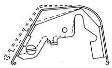
NOTE: Caution should be used while forming to prevent possible contact of the rear edge of the paper table with the margin set finger.
