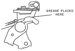
3. Using a spring hook or similar tool, apply a very small amount of #17 grease to the area where the trip lever contacts the cam. Care should be exercised not to over-lubricate, as this could result in possible migration of grease to the power roll. When lubricating a complete set of cams in this manner, it is recommended that the cam knockoff bar be removed (Standard ET) to facilitate lubrication.
