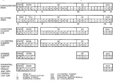
Figure 2 Configuration- and selection-mask formats and configuration contents
