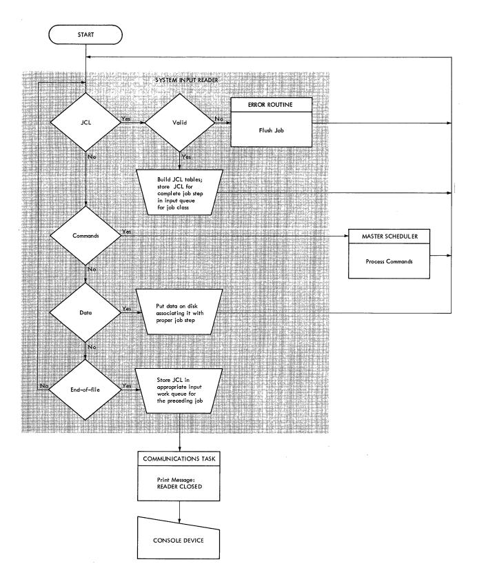
Figure 18. System Input Reader Processing
