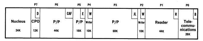
Figure 24. Sample 256K Telecommunications, CPO, and Batch Processing Configuration
