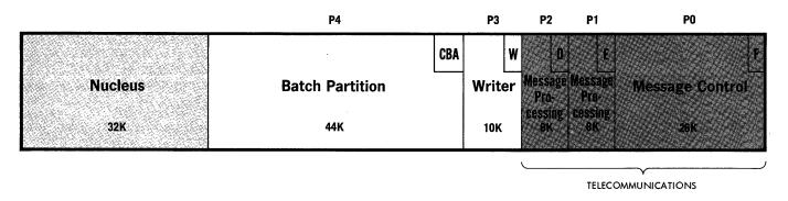
Figure 22. Sample 128K Telecommunications-Oriented Configuration
