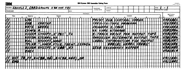
Figure 33. Job Control and Program Control Statements for Card-to-Tape Job
