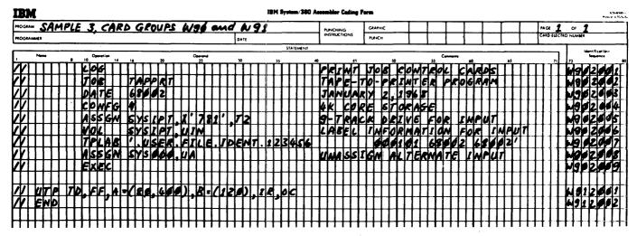
Figure 35. Job Control and Program Control Statements for Tape-to-Printer Job (Unsorted Records)
