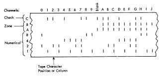
Figure 1. Magnetic Tape Data in the BCD Code
