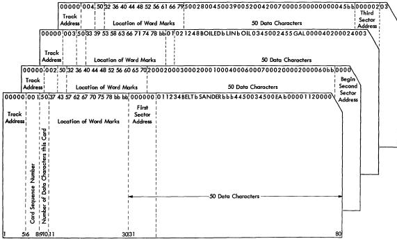
Figure 6. Disk-to-Card Example -- Load Mode
