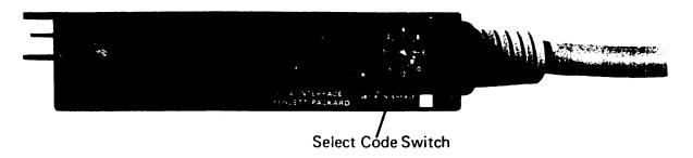
Figure 2-1 Interface Card Select Code Switch
