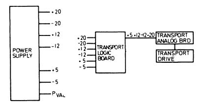
Figure 4-3. Power Supply Block Diagram
