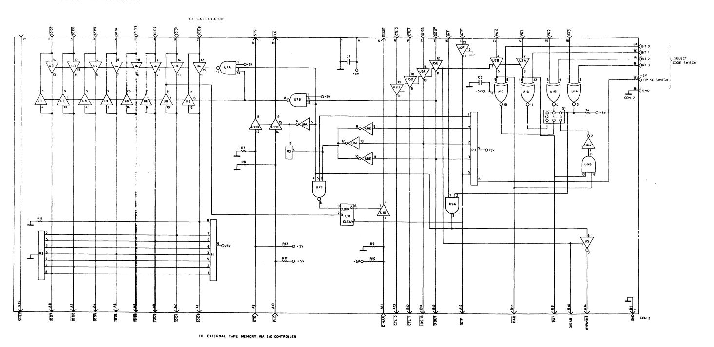
FIGURE 6-5 A1 Interface Board Assembly Schematic Diagram
