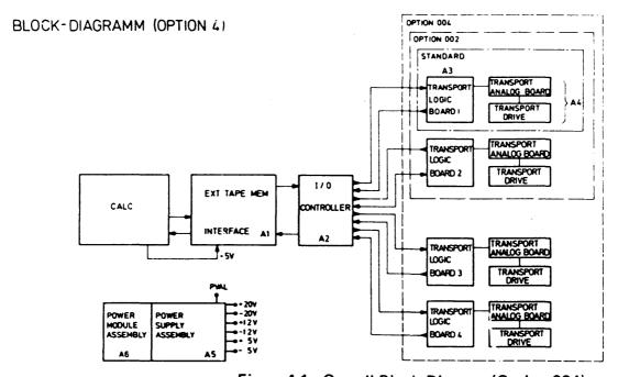
Figure 4-1. Overall Block Diagram (Option 004).
