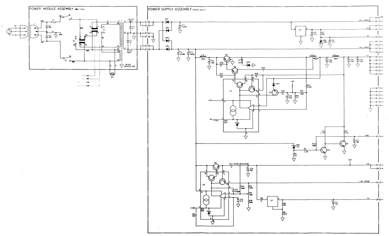
FIGURE 6-4 A5 Power Supply Assembly Schematic Diagram
