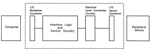
Figure 2-1. Interface Functional Diagram
