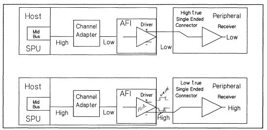
Figure 2-22. Single-Ended Cabling to External Device
