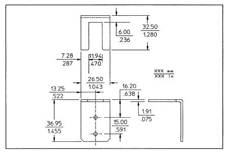
Figure 2-17. A Cable Grounding Bracket
