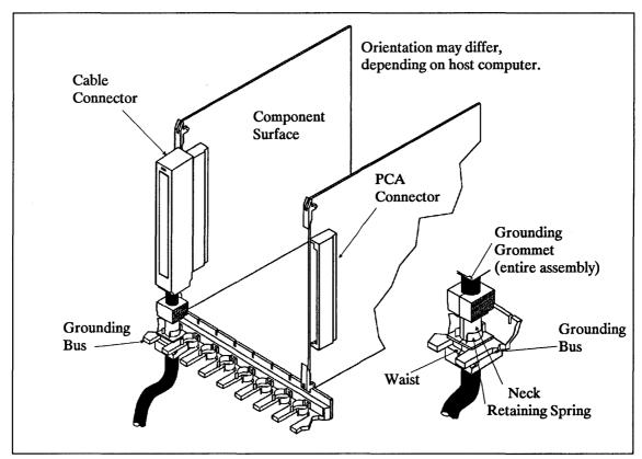
Figure 2-16. A Typical AFI Installation
