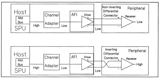
Figure 2-21. Differential Wiring for External Device Connector
