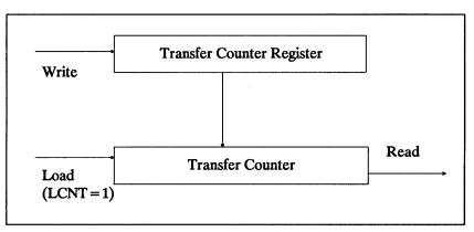
Figure 3-2. Transfer Counter Operation
