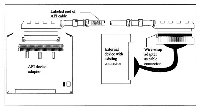
Figure 2-20. The Wire-Wrap Adapter in an Intermediate Cable
