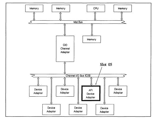
Figure 1-2 is a block diagram showing a typical HP computer system with an AFI installed.
