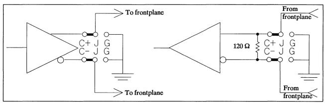
Figure 2-10. Driver/Receiver Connection in Differential Mode
