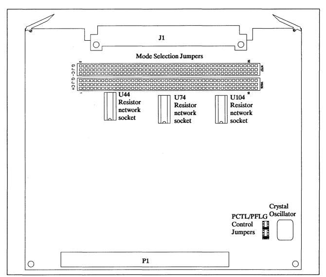
Figure 2-1. Locations of Configuration Jumpers
