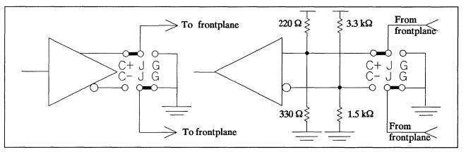
Figure 2-4. Driver/Receiver Grounding in Single-Ended, High-True Mode
