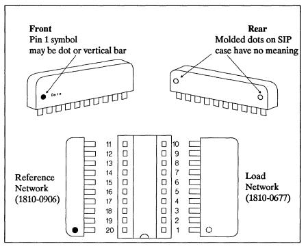
Figure 2-3. Installing the High-True Resistor Network SIPs
