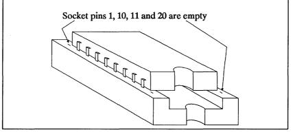
Figure 2-9. Installing the Differential Resistor Network DIPs
