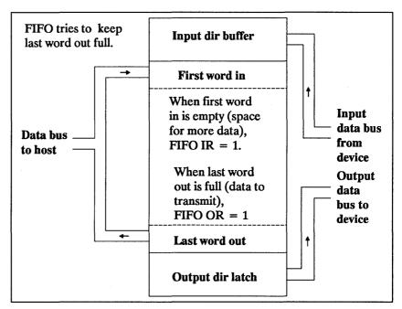
Figure 3-11. FIFO Buffer Signals IR and OR
