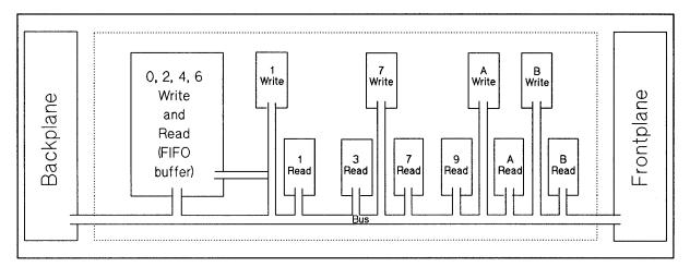
Figure 3-3. AFI Registers on the Data Bus
