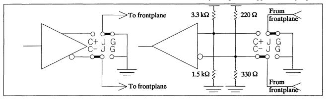
Figure 2-7. Driver/Receiver Grounding in Single-Ended, Low-True Mode
