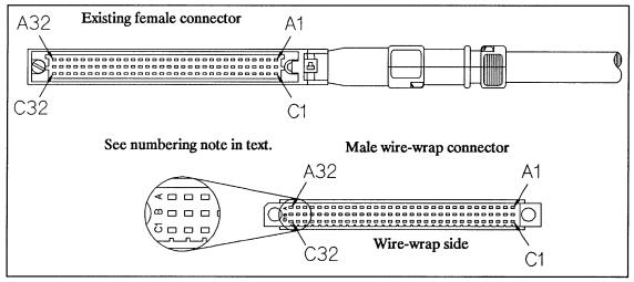
Figure 2-18. The Wire-Wrap Pinout Orientation
