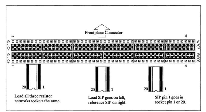
Figure 2-5. Single-Ended, Low-True Configuration
