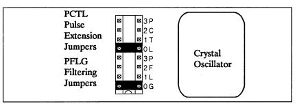
Figure 2-11. Output Control Jumpers
