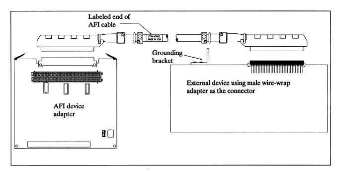
Figure 2-19. The Wire-Wrap Adapter as the External Device Connector
