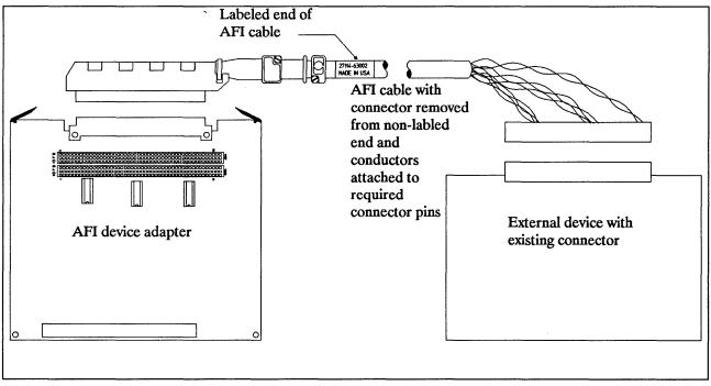
Figure 2-15. Wiring the Custom AFI Cable
