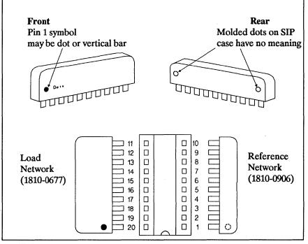
Figure 2-6. Installing the Low-True Resistor Network SIPs
