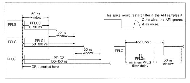
Figure 2-13. Examples of PFLG Filter Accepting and Rejecting Signal
