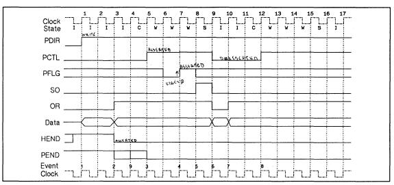
Figure 3-5. Output FIFO Handshake
