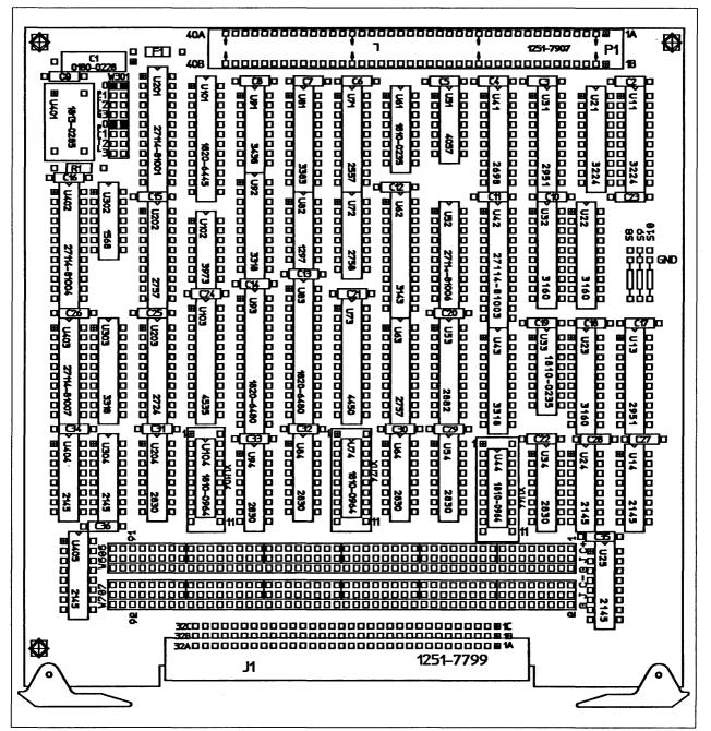
Figure D-1. AFI Parts Location Diagram
