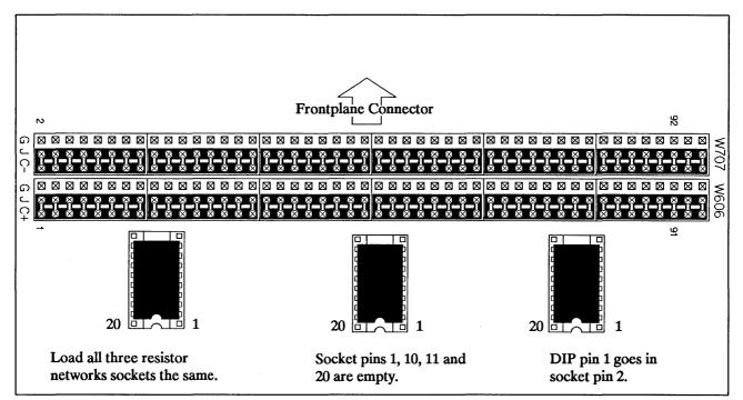
Figure 2-8. Differential Mode Configuration
