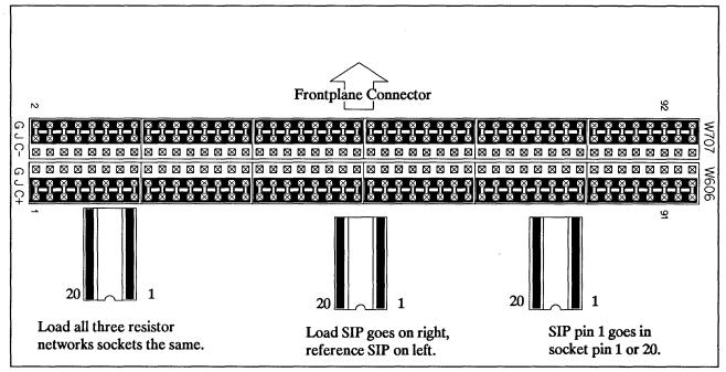
Figure 2-2. Single-Ended, High-True Configuration
