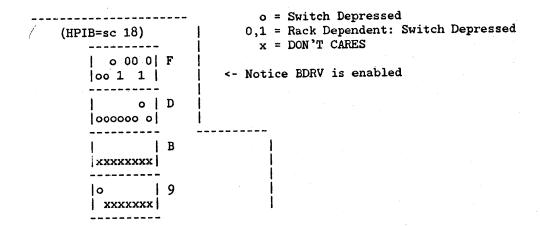
The 98206 card has been equipped with a toggle switch. For normal operation the switch should be toggled to the 'LEFT' (away from the Red LEDs). During some tests the operator may be directed to disable the card by toggling the switch to the 'RIGHT.' Always remember to switch it back after completing the tests.
