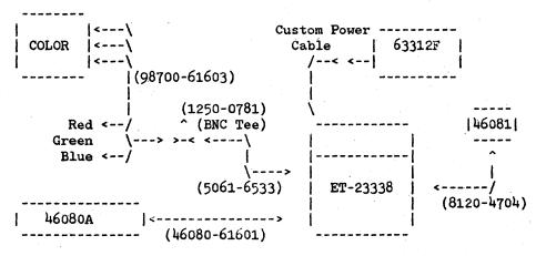
Please notice that the above layout illustrates the suggested arrangement with a color monitor. A 35721A type display would use a #8120-4704 cable to the UUT instead of what is shown.
