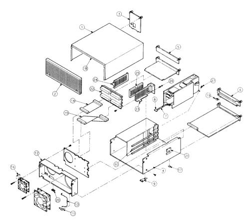
Figure 8-2. Model 332 Computer Case Parts
