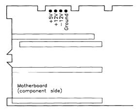
Figure 4-1. Power Supply Test Points
