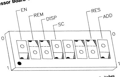
Figure 3-2. Processor Board Configuration Switches
