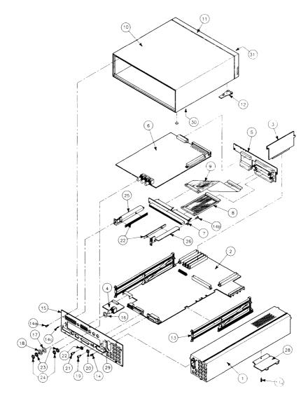
Figure 8-1. SPU Exploded View
