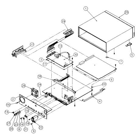
Figure 8-1. SPU Exploded View
