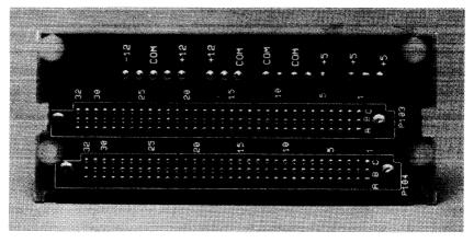
Figure 4-1. Power Supply Test Points
