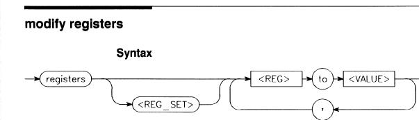
**Function** The modify register command is used to modify the contents of one or more registers in the processor/corpocessor's register set. The entry for <REG> determines which register is modified.
