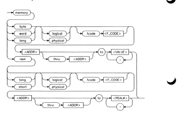
**Function** The modify memory command enables you to modify the contents of selected memory locations. The command can modify the contents of each memory location in a series to an individual value or the contents of all of the locations in a memory block to a single or repeated sequence of values.
