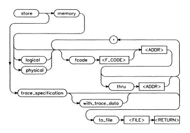
**Function** The store command is used to store the contents of specific memory locations into an absolute file (.X file), or to store the trace specification, with or without trace data, into a trace file (.TR file).
