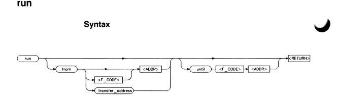
**Function** If the processor is in a reset state, run will cause the reset to be released, and if a **"from**" address is specified the processor will be directed to that address. If the processor is running in the monitor, the run command causes the processor to exit into your program. The program can either be run from a specified address (--EXPR--), from the address currently stored in the program.
