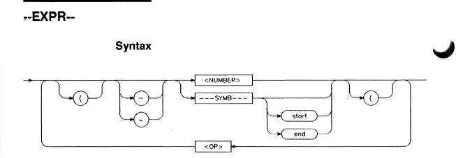
**Function** An expression is a combination of numeric values, symbols, operators, and parentheses specifying an address, data, status, or any of several other value types used in the emulation commands.
