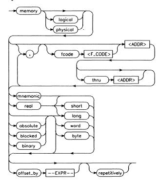
**Function** The display memory command displays the contents of the specified memory location or series of locations. The memory contents can be listed in mnemonic, binary, hexadecimal, or real number format. In addition, the memory addresses can be listed offset by a value which allows the information to be easily compared to the program listing.
