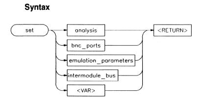
**Function** The set command is used to change the configuration for analysis, the bnc ports, or the intermodule bus; to modify emulation timeout; or to set up environmental variables.
