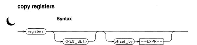
**Function** The copy registers command copies the current contents of the processor/coprocessor's various register sets. This process does not occur in real time. The emulation system must be configured for nonreal-time run mode if the registers are to be listed while the processor is running.
