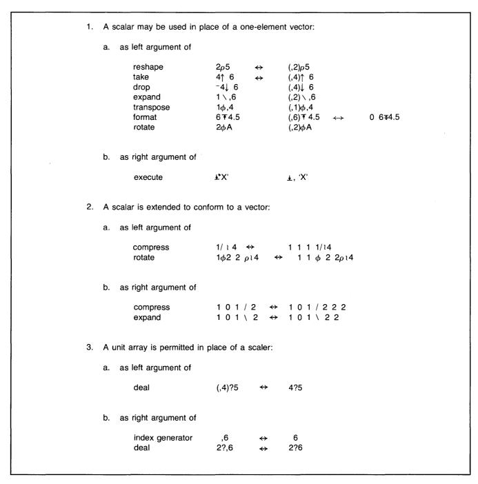
Figure 3-2. Scalar-Vector Substitutions for Mixed Functions
